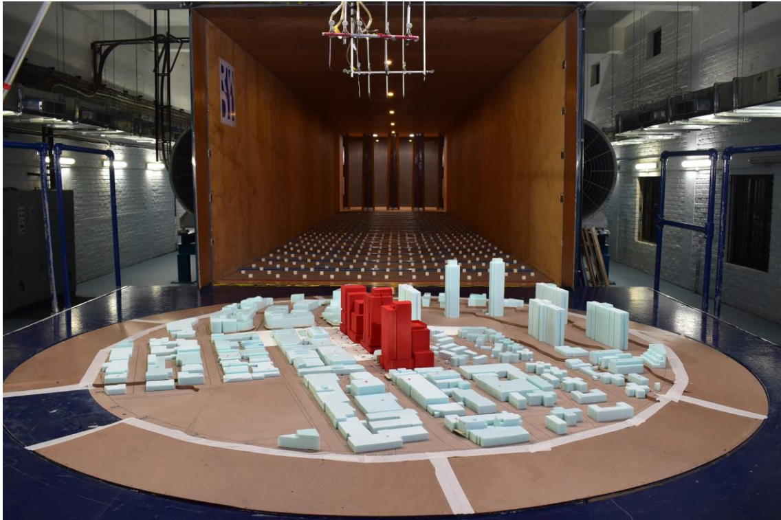
Figure A-1 – Wind Tunnel Model of Amended Design Scheme (View from South)
