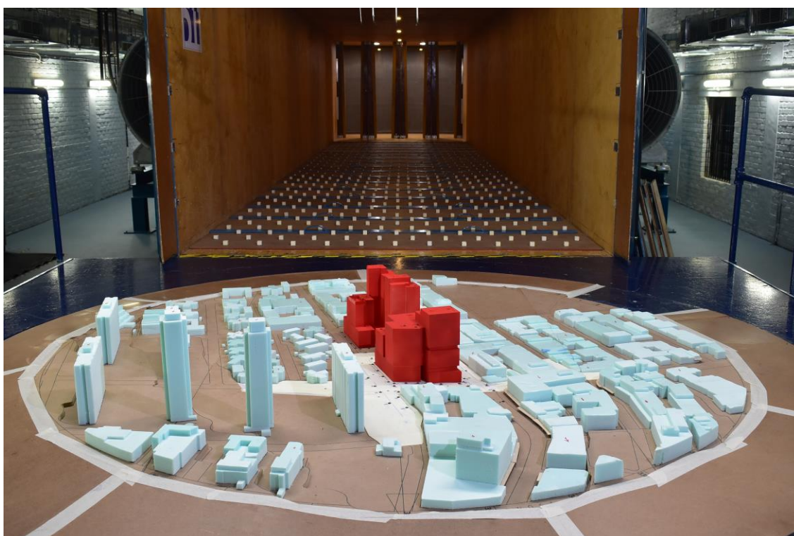
Figure A-4 – Wind Tunnel Model of Amended Design Scheme (View from North)
