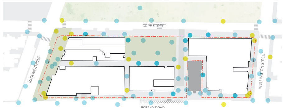
Reference Design Proposal including mitigation Ground Level Wind Tunnel Results – Summer Period
