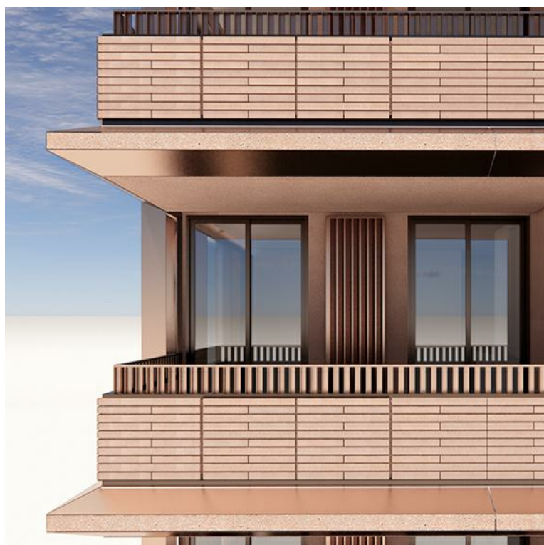
BT-02 Solid-Metal Balustrade Solid upstand with small format terracotta panels in matt and glazed finish. Aluminium balustrade above. Powdercoat 'metallic' finish Colour - 'copper/bronze'
