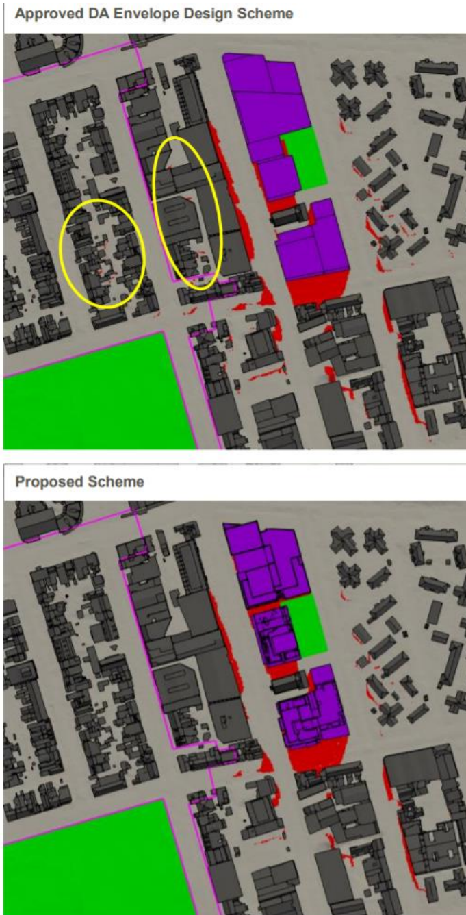
Figure 54 Comparison of approved concept DA and proposed development of grade level areas where direct solar access is reduced to less than two hours on 21 June
