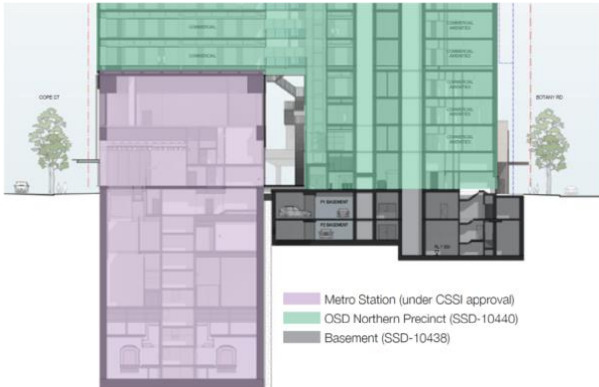
Figure 17 E-W Section view illustrating the relationship of the metro station box and basement
