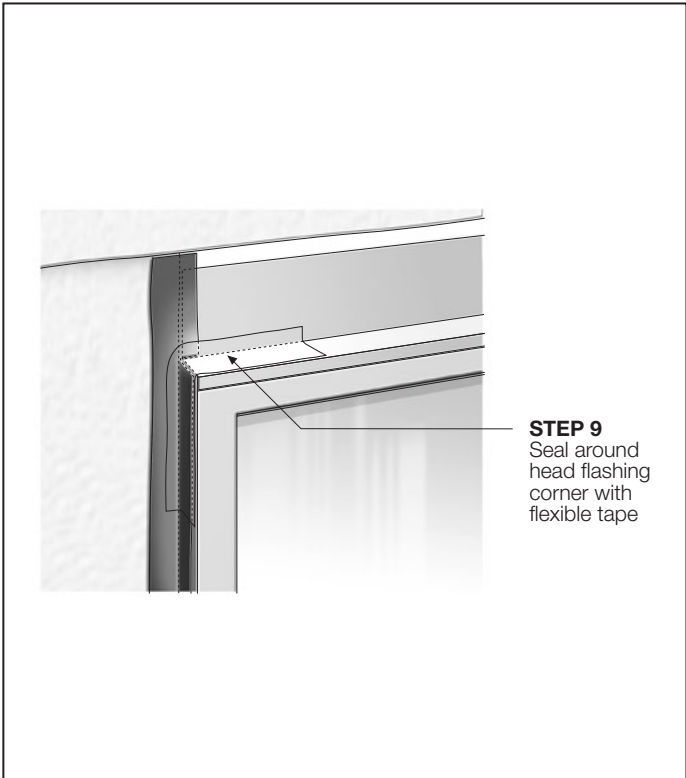
FIGURE 46 INSTALLATION OF WINDOW
