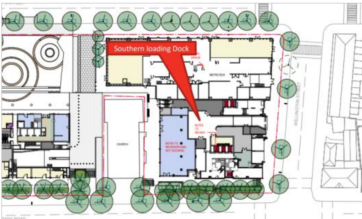
Figure 27 Vehicular access to Southern Loading Dock
