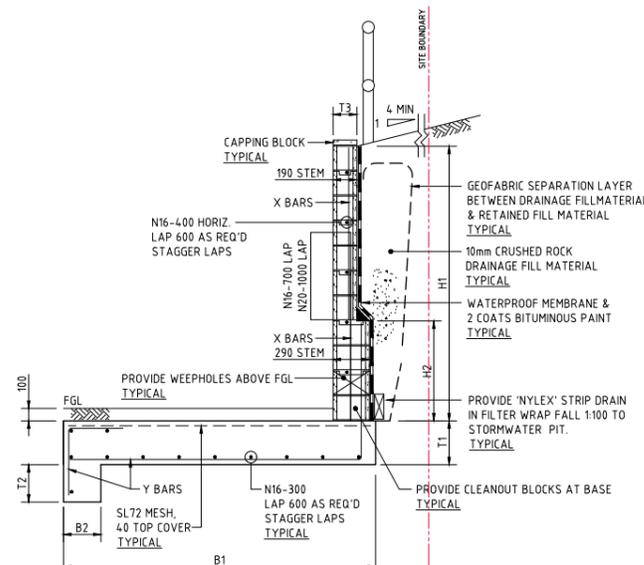
WALL WITH THIN STEM OF 190 BLOCK AND THICK STEM OF 290 BLOCK
