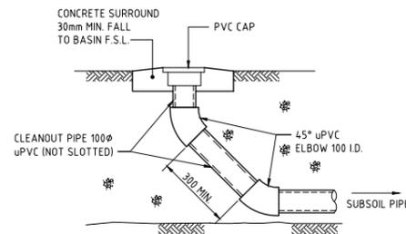
**BIO-RETENTION CLEANOUT EYE ELEVATION**
