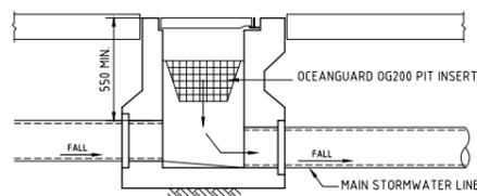
**Stormwater Pit with EnviroPod Configuration**
