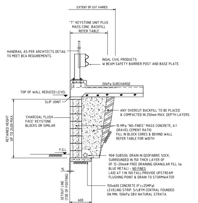
'NO-FINES' MASS CONCRETE KEYSTONE RETAINING WALL
