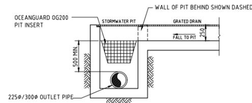
**Grated Drain/Stormwater Pit with EnviroPod Configuration**
