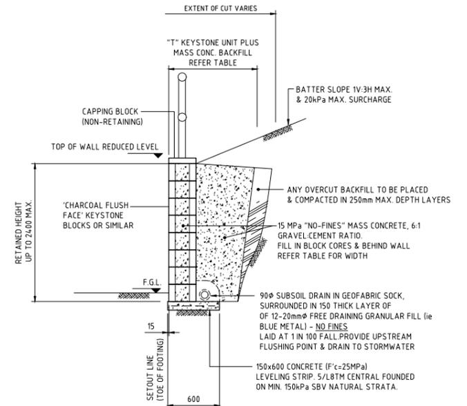
'NO-FINES' MASS CONCRETE KEYSTONE RETAINING WALL
