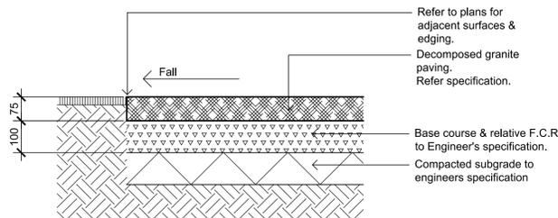
04 DG - Decomposed Granite Paving on Grade
