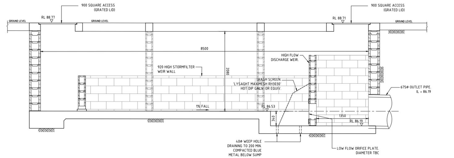
SECTION 1:20 1 : TYPICAL THRU' TANK
