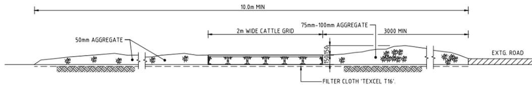
**SECTION 1:20 1 : STABILISED CONSTRUCTION ENTRANCE 'TRUCK SHAKER'**
