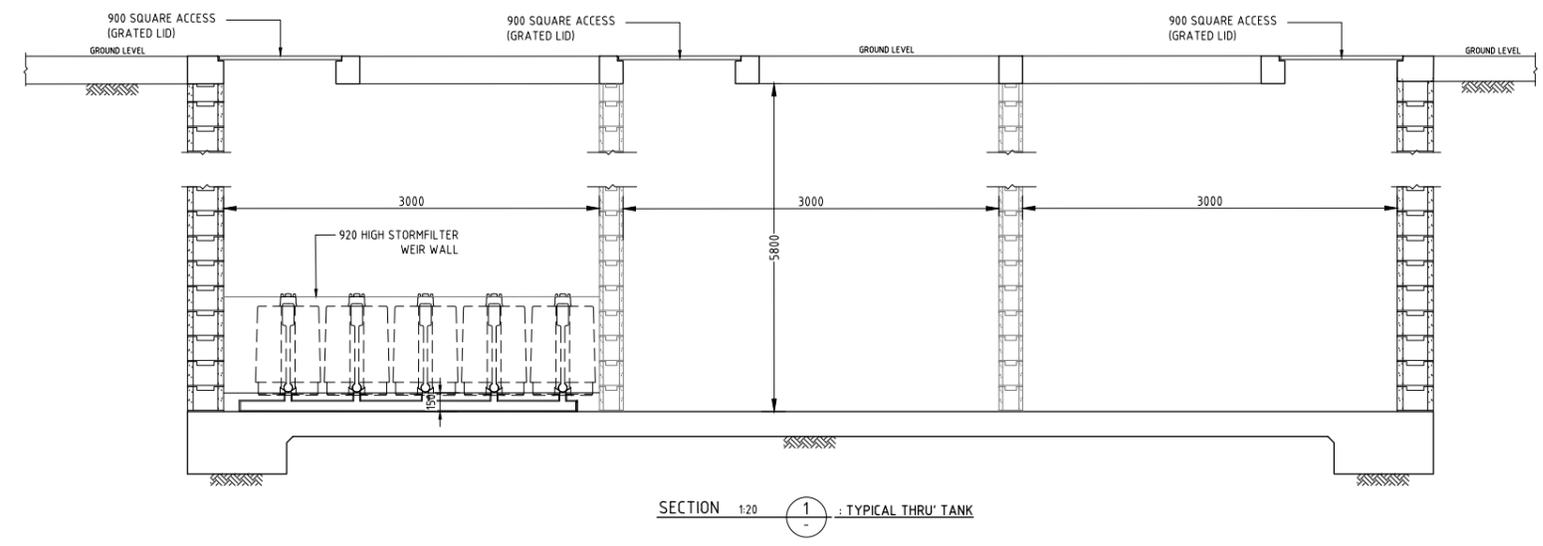
SECTION 1:20 : TYPICAL THRU' TANK
