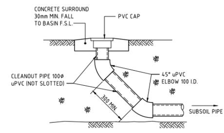
**BIORETENTION CLEANOUT EYE ELEVATION**
