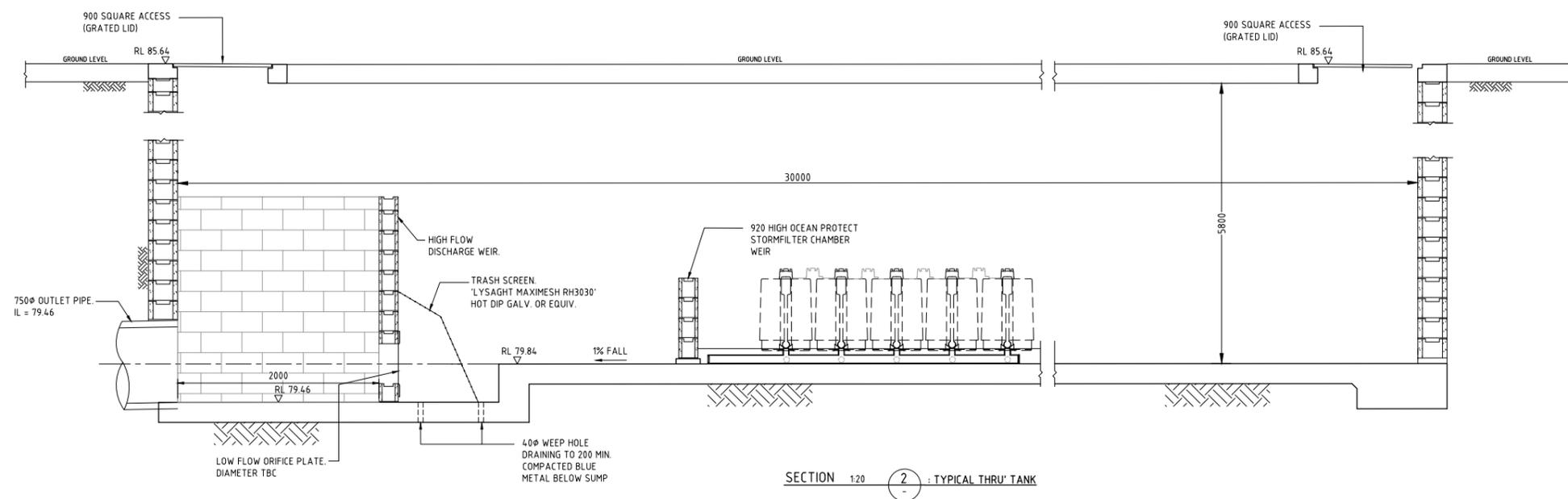
SECTION 2:20 : TYPICAL THRU' TANK
