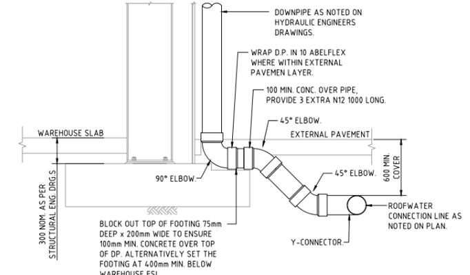
**DOWNPIPE TURN-UP DETAIL A (AT FOOTING LOCATION)**
