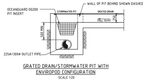
**GRATED DRAIN/STORMWATER PIT WITH ENVIROPD CONFIGURATION**
