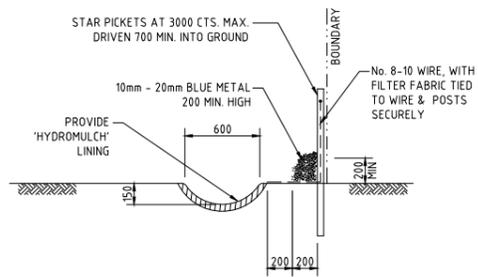
**TYPICAL OPEN DRAIN & SILT FENCE**
