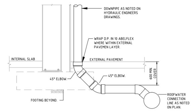
**DOWNPIPE TURN-UP DETAIL B (CLEAR OF FOOTING)**
