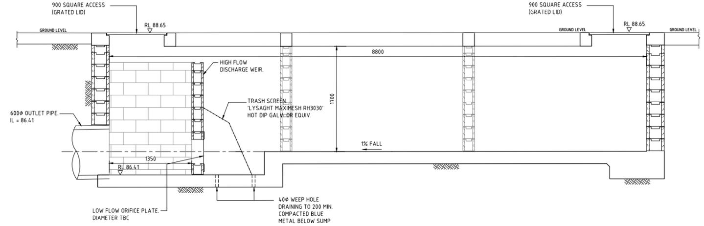
SECTION 120 1 : TYPICAL THRU TANK
