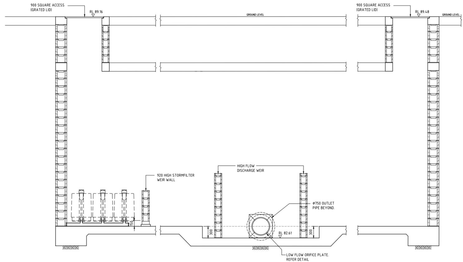
SECTION 1-1 : TYPICAL THRU' TANK
