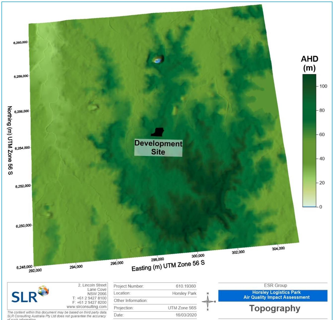
The overall elevation of the Development Site ranges from approximately 60 m to 80 m Australian Height Datum (AHD) with the quarry pit and stockpiles contributing to the complexity of the terrain within the site. This will be graded and levelled as part of the construction works. The Development Site is located on a ridge, with potential for light air drainage flows along the north-south channel, under calm conditions.
