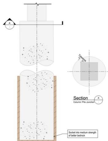
Figure 3: Typical Bored Pile Section & Plan
