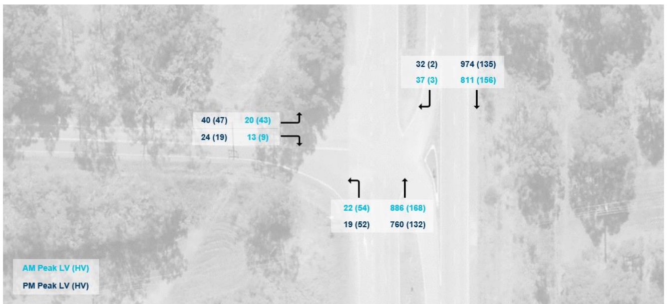
Figure 5.4 Italia Road / Pacific Highway – Future traffic volumes (2032 volumes + quarry generated volumes)
