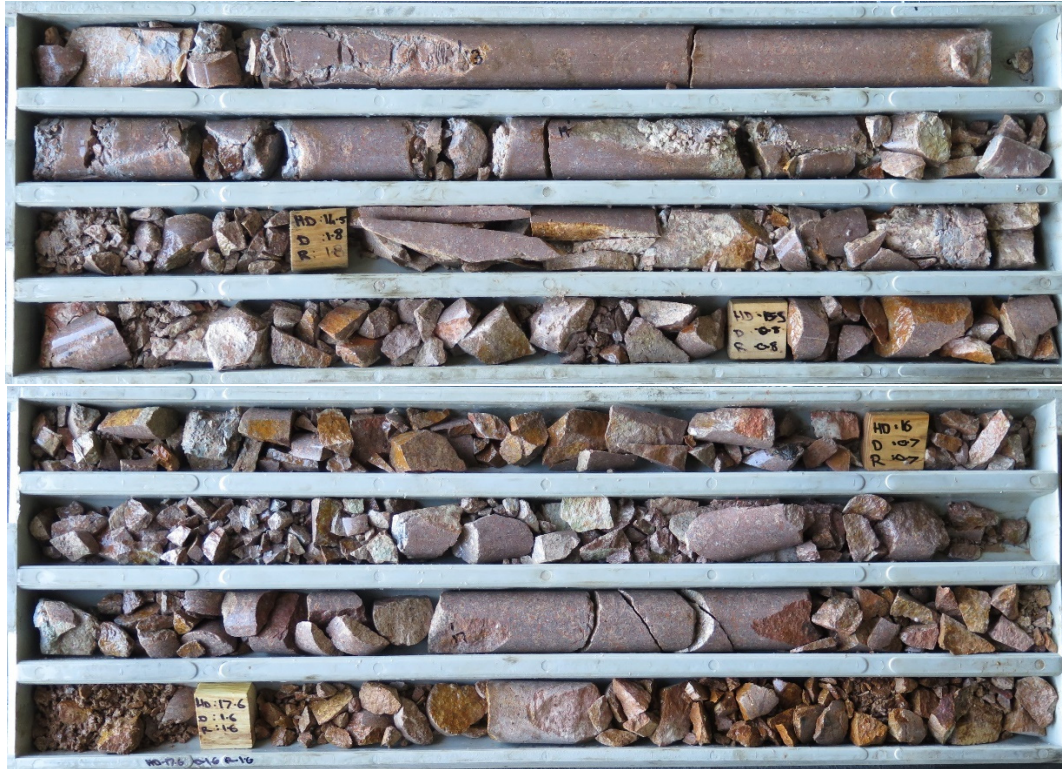
Plate 28 – Intensely fractured rhyodacite associated with the Central Fault – drill hole ARDG-DDH05 (12.75-18.00 m).
