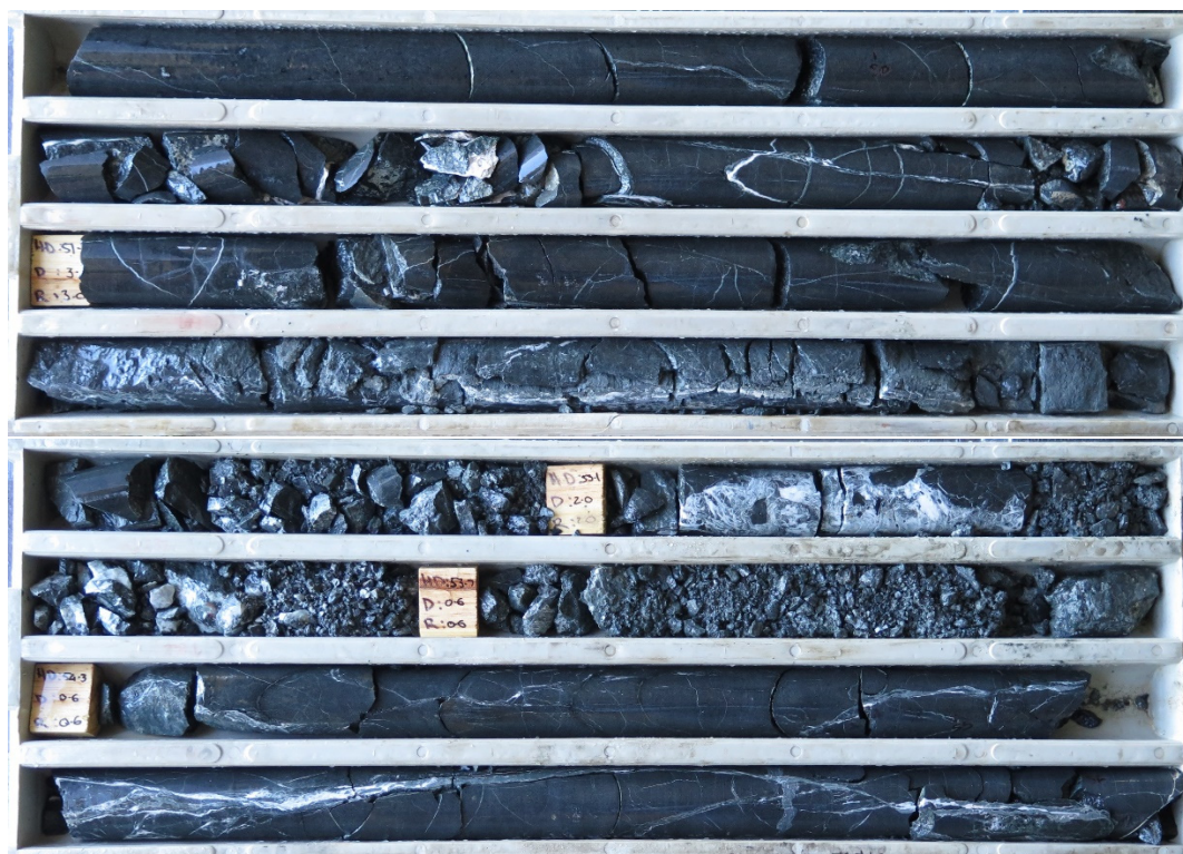
Plate 29 – Intensely fractured, brecciated and calcite veined dolerite within the Central Fault – drill hole ARDG-DDH05 (49.40-55.90 m).
