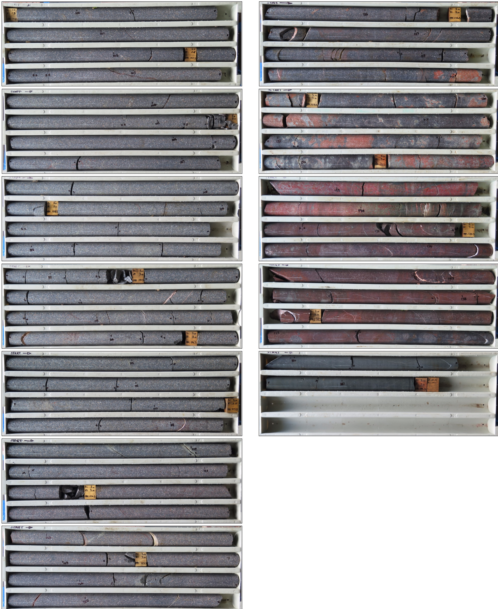
Plate 22 (continued) – Typical intersection through rhyodacite of the middle stratigraphic sequence – diamond drill hole ARDG-DDH16
