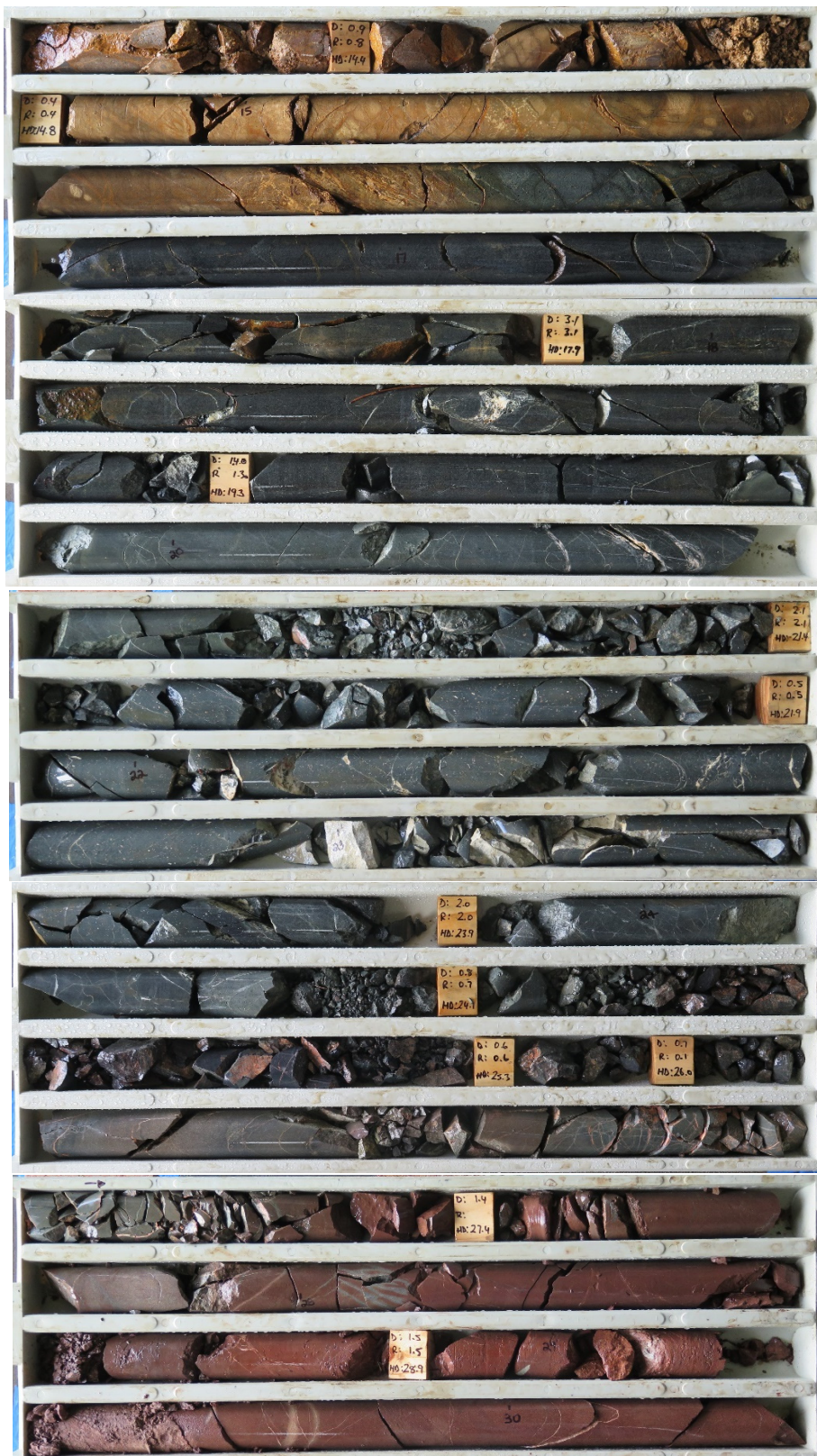
Plate 31 – Strongly to intensely fractured dolerite dyke at contact between clay-altered lithic sandstone and hematitic sedimentary units within the Nine Mile Creek Fault Zone – drill hole ARDG-DDH20 (14.15-30.30 m).
