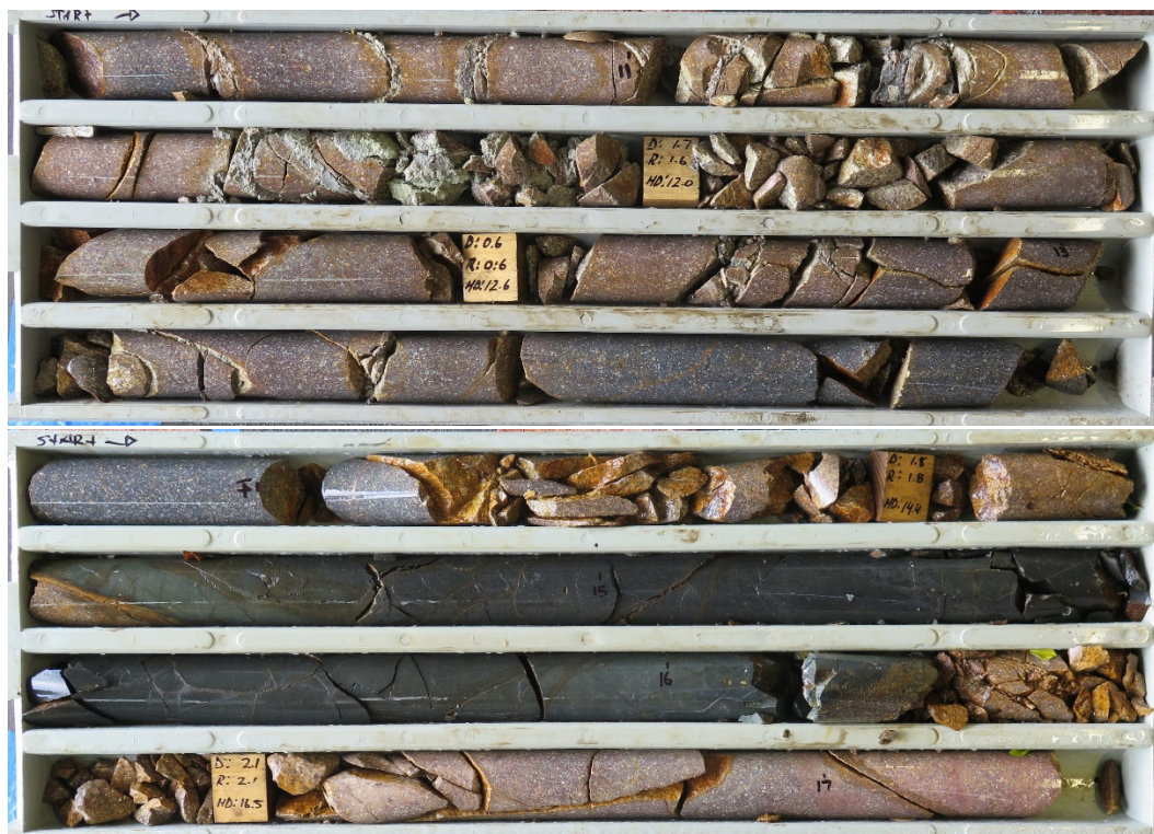
Plate 30 – Strongly fractured rhyodacite and a narrow dolerite dyke associated with the Central Fracture – drill hole ARDG-DDH16 (10.60-17.20 m).
