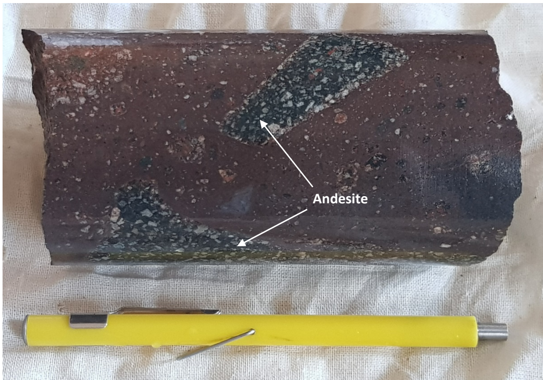
Plate 13 – Coarse volcanic breccia containing fragments of porphyritic pyroxene andesite – drill hole ARDG-DDH08 (36.29-36.41 m).
