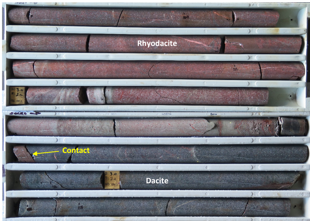
Plate 23 – Contact between rhyodacite and underlying dacite in drill hole ARDG-DDH15 (108.50-115.70 m). This contact occurs north of the Central Fault. The rhyodacite is pervasively altered by hematite ± laumontite.
