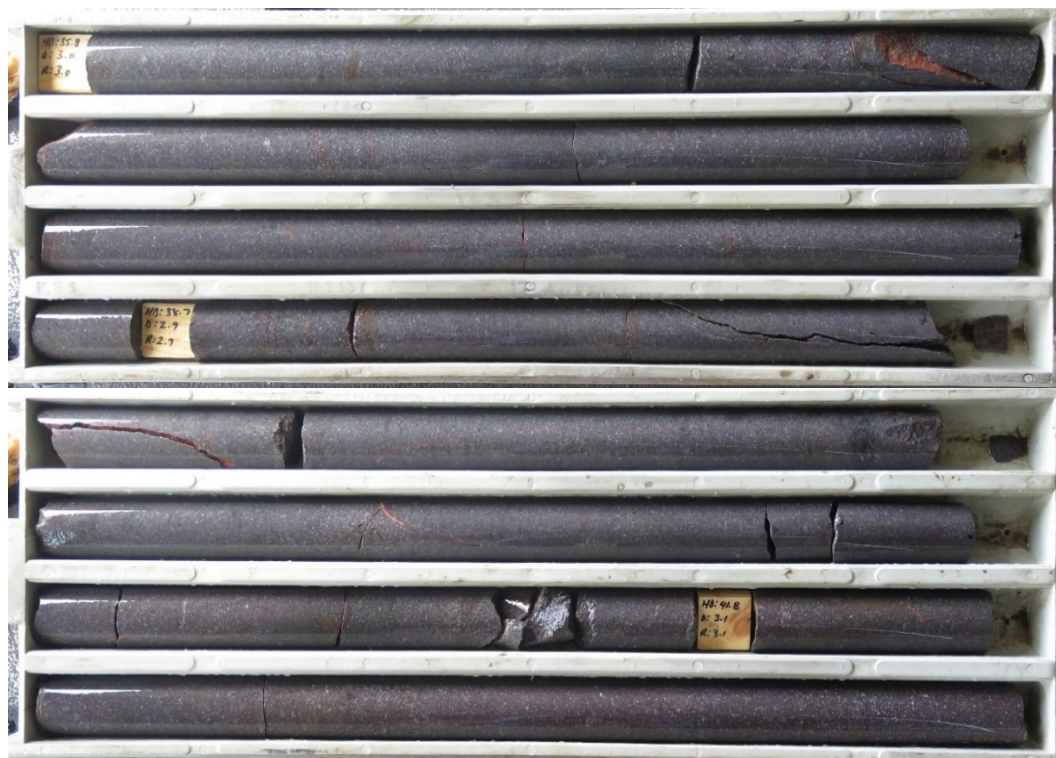
Plate 17 – Massive unfractured dacite – drill hole ARDG-DDH03 (35.80-43.00 m).
