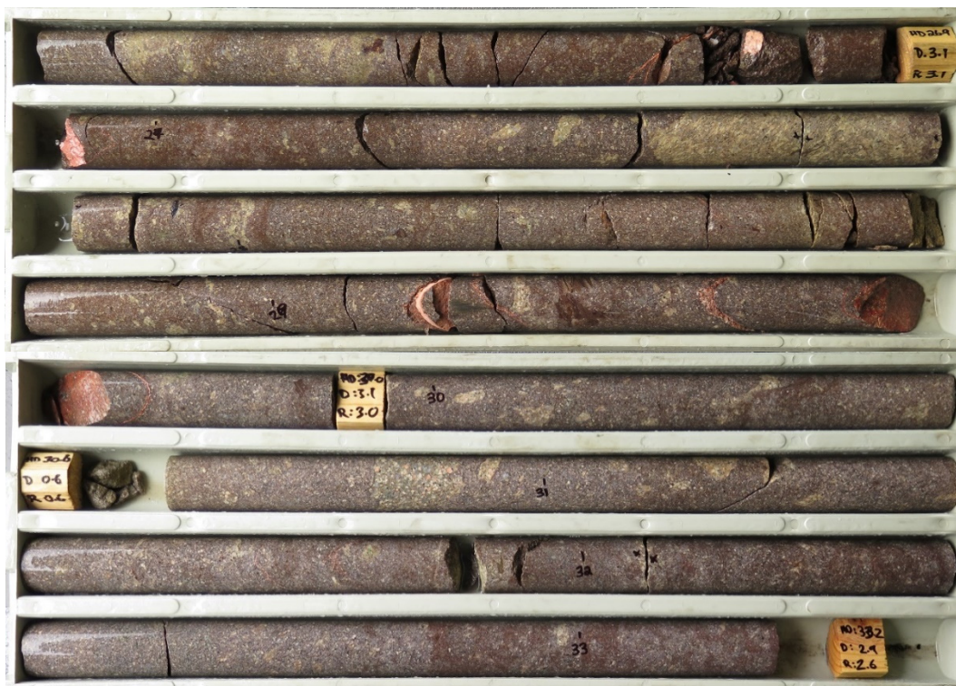
Plate 25 – Crystal-vitric-lithic tuff of rhyodacitic composition – drill hole ARDG-DDH06 (26.10-33.20 m). The pale cream-green colour is predominantly related to alteration by sericite.
