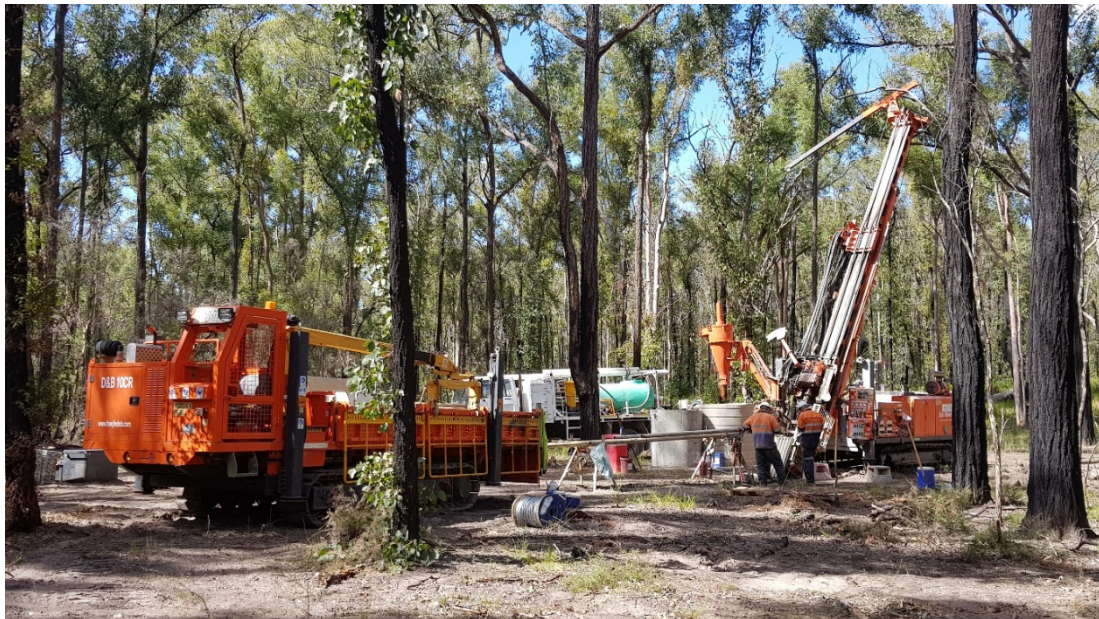
Plate 10 – Hanjin D&B-35 Multi drill rig with Hanjin 10CR track-mounted rod carrier (foreground). Drill hole ARDG-DDH06 – April 2018
