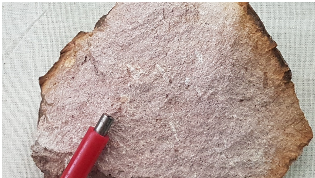
Plate 5 – Altered vitric-crystal welded tuff of rhyodacite composition from outcrop south of Stone Ridge (Sample H2)
