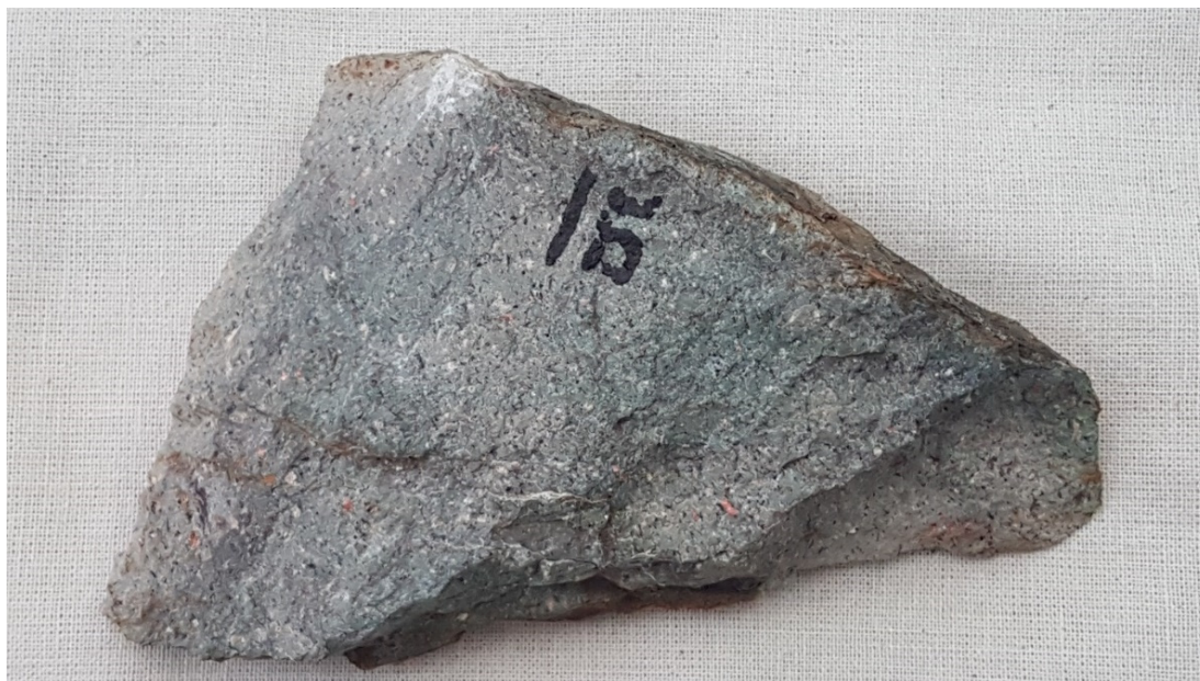
Plate 6 – Vitric-crystal welded tuff of rhyolite composition from outcrop north of Stone Ridge (Sample 15)
