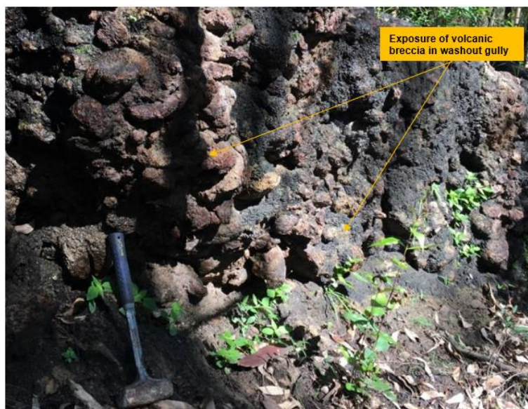
Figure 2.7 Volcanic Breccia in washout gully on Stone Ridge (Provided by Australian Resource Development Group)
