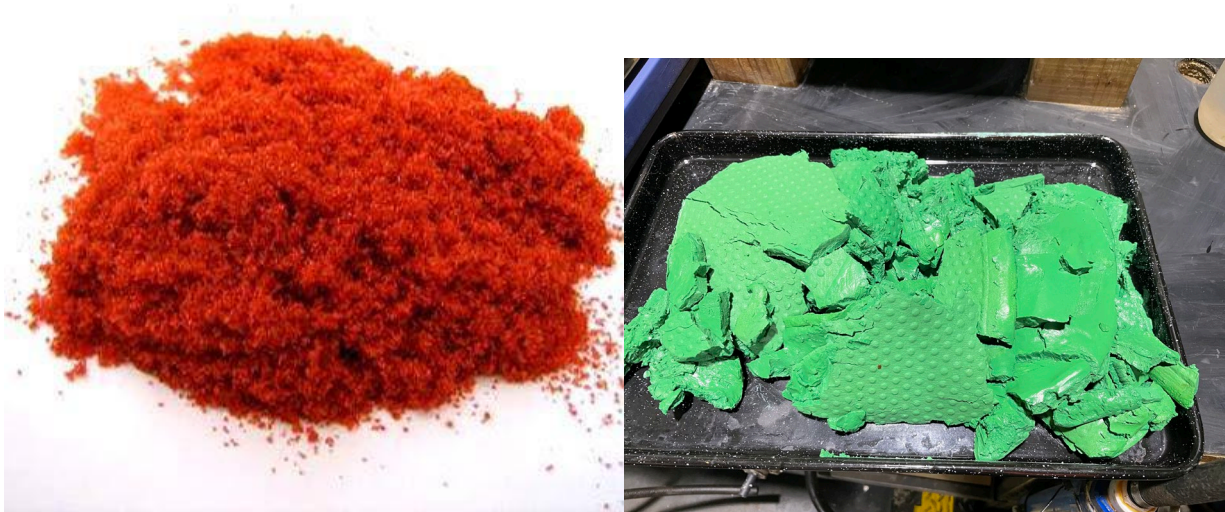
Figure 14: Cobalt sulphate heptahydrate (red) and Mixed Metal Hydroxide (green)
