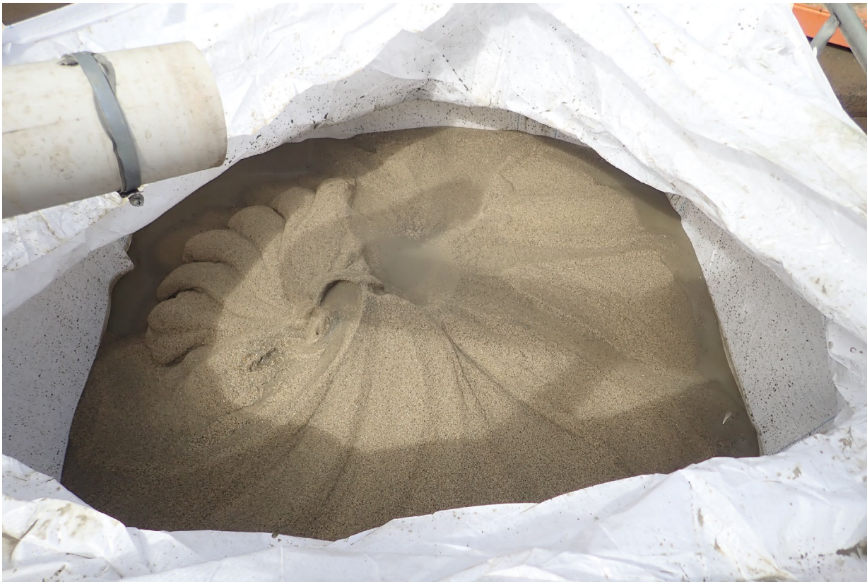
Figure 19: Coarse reject generated from comminution test work.
