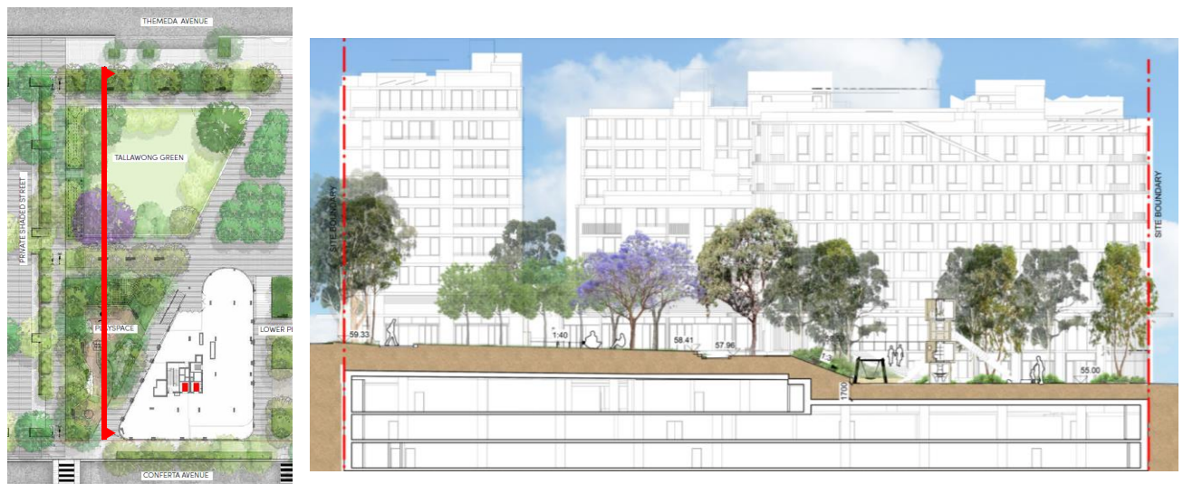
Figure 17 | North-south section through park in Site 1 showing deep soil zone over basement (Source: Applicant's EIS)
