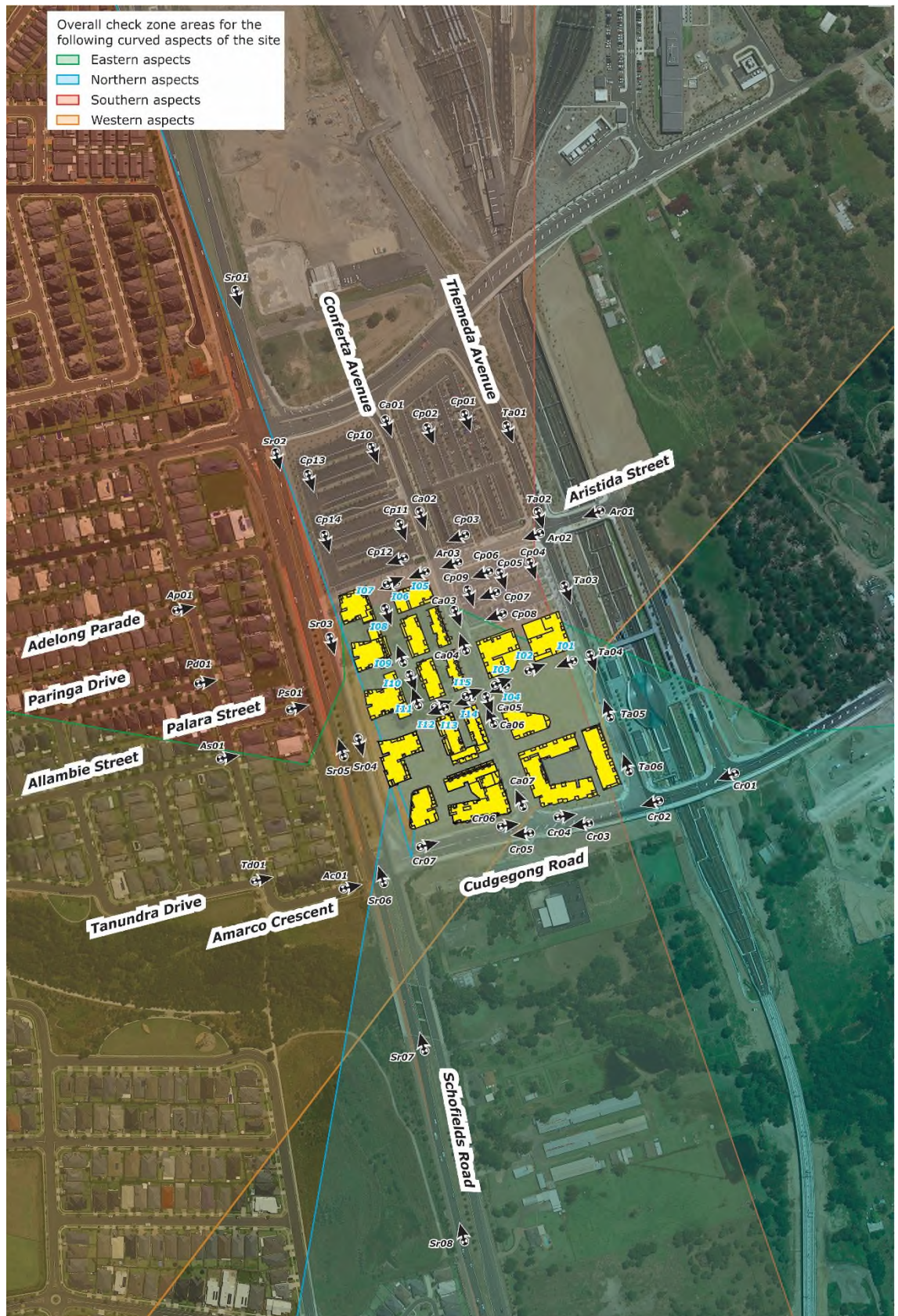
Figure 2a: Check Zones and Study Point Locations – Flat Aspects (the check zones are the areas where glare could potentially be observed)
