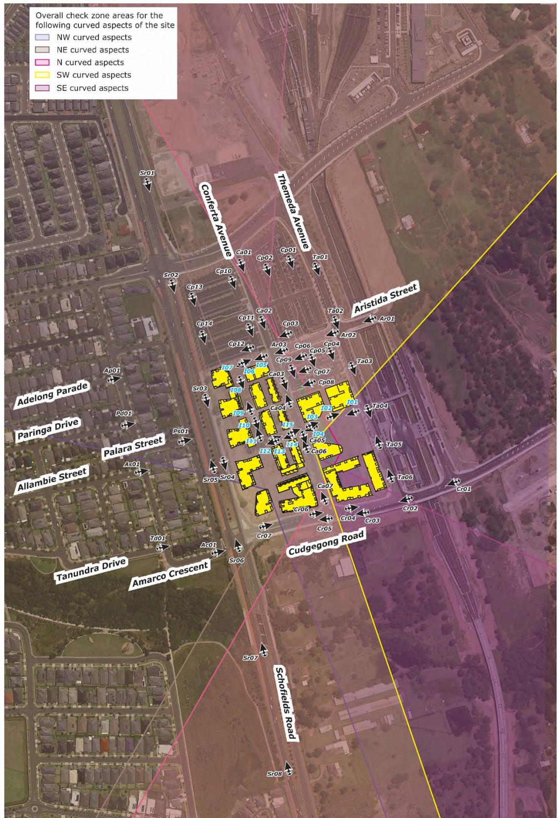
Figure 3b: Check Zones and Study Point Locations – Curved Aspects (the check zones are the areas where glare could potentially be observed)
