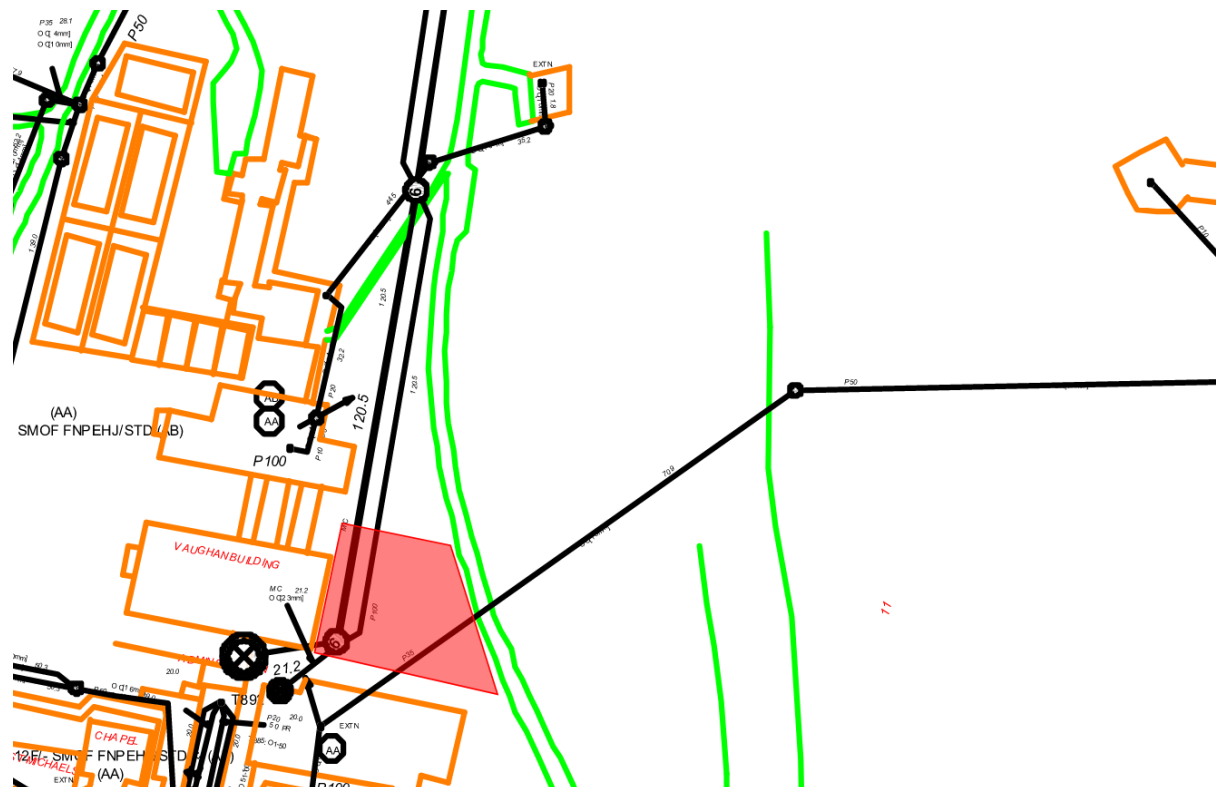
Extract from Telstra survey plan showing conduits traversing site (highlighted in red)
