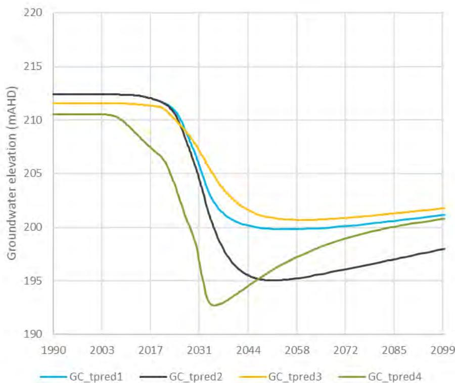
**Figure D.3 Modelled groundwater elevation hydrograph at water supply work GW803422**
