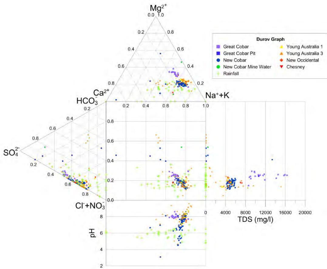
**Figure 3.5** Major ion concentrations (as meq/L) for Cobar groundwater samples
