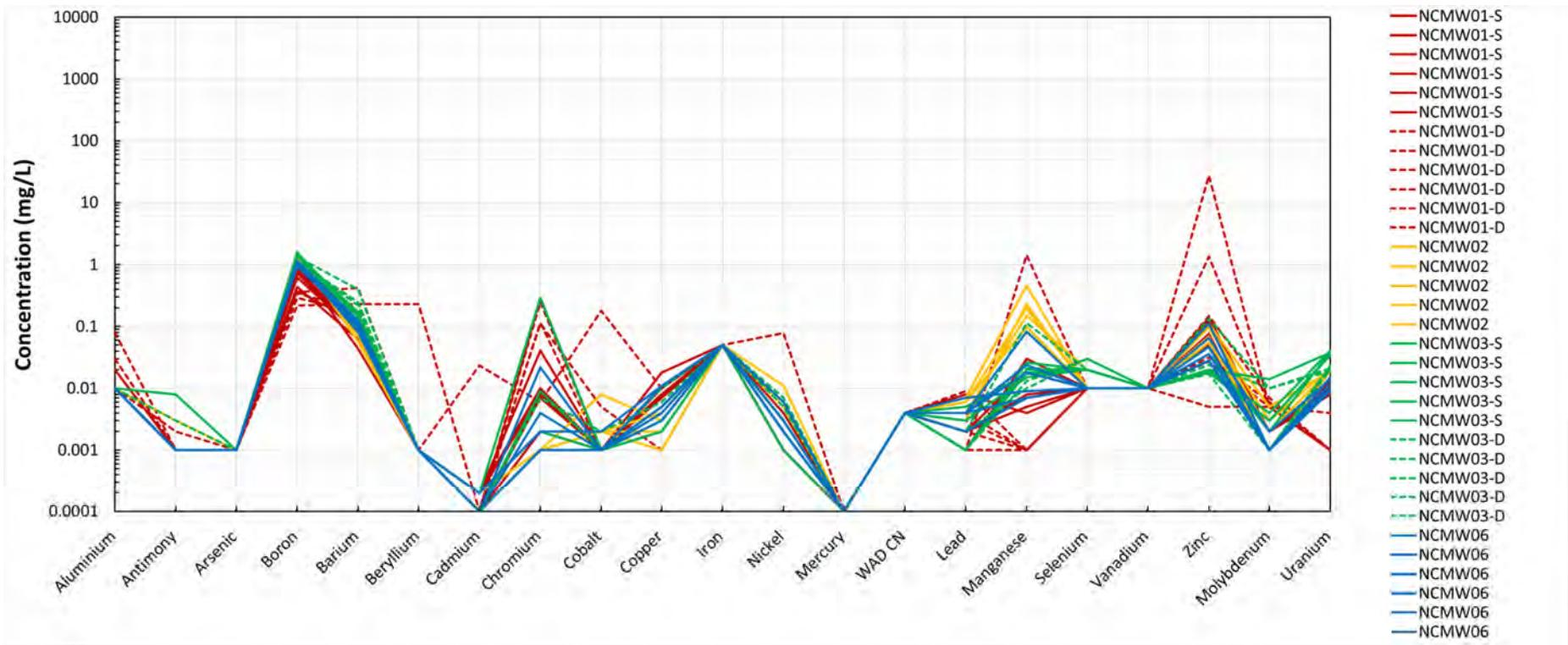
**Figure 3.7** Metal/metalloid concentrations of New Cobar Complex groundwater monitoring bores
