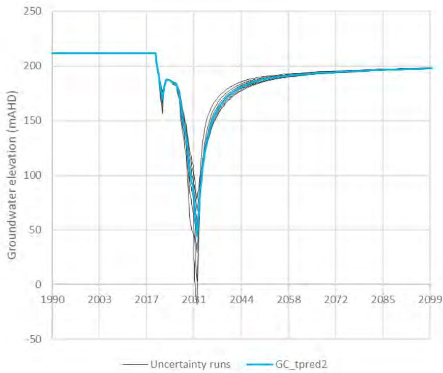
**Figure D.6** Great Cobar shaft modelled mine void uncertainty analysis groundwater elevation hydrograph
