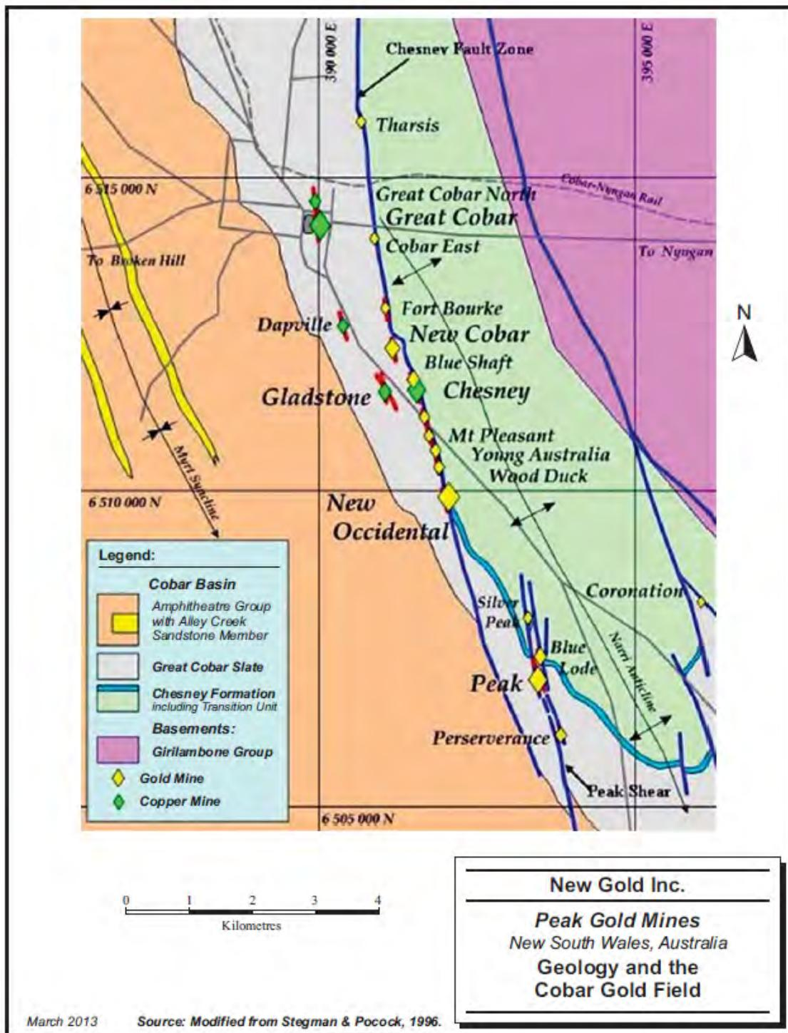
Figure 3.1      Simplified Cobar geology
