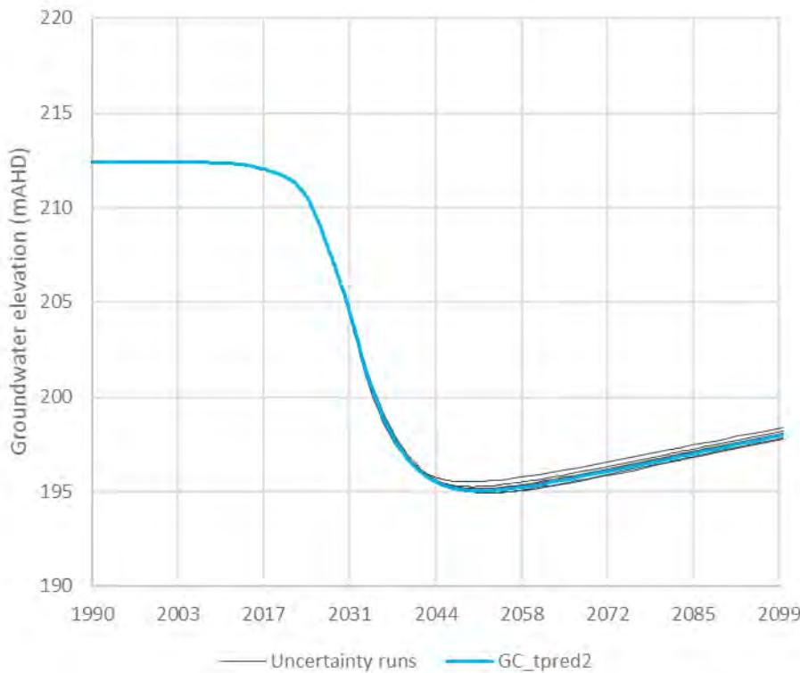
**Figure D.4      Rugby club bore modelled mine void uncertainty analysis groundwater elevation hydrograph**
