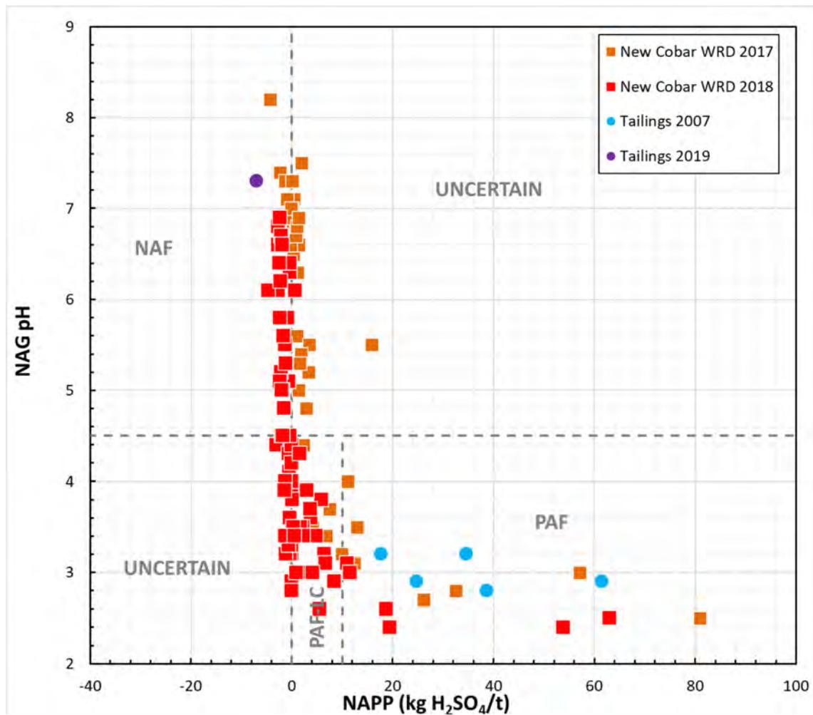
**Figure 3.4** NAPP versus NAG pH for Cobar waste material
