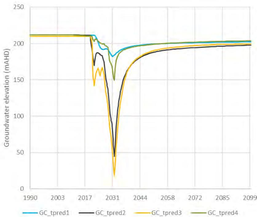
**Figure D.5** Great Cobar shaft modelled groundwater elevation hydrograph
