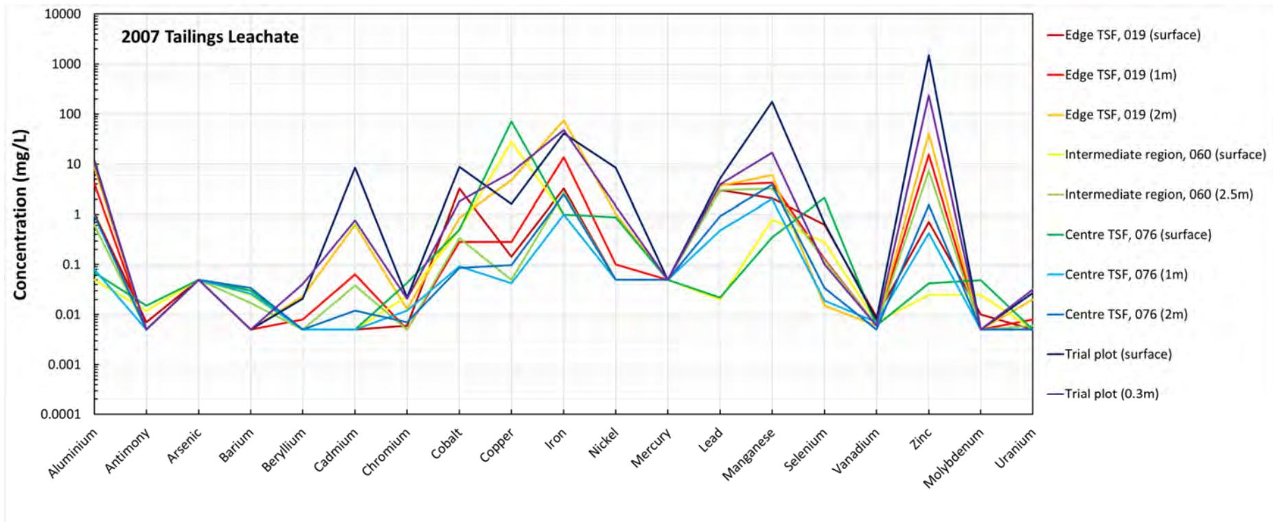
Figure 3.10 Peak Complex tailings samples and leachate testing concentrations
