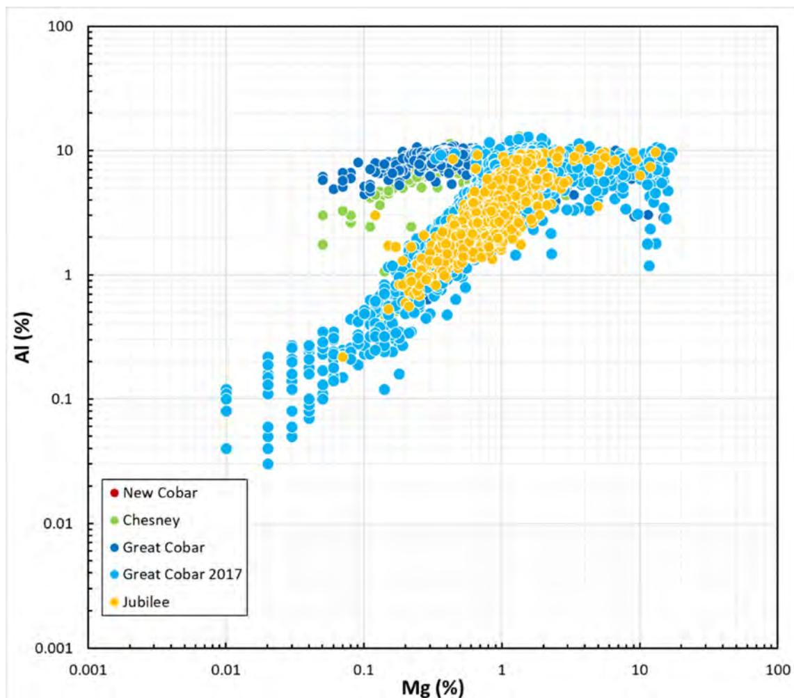
**Figure 3.3 Major element magnesium versus aluminium for New Cobar Complex ore body assays**
