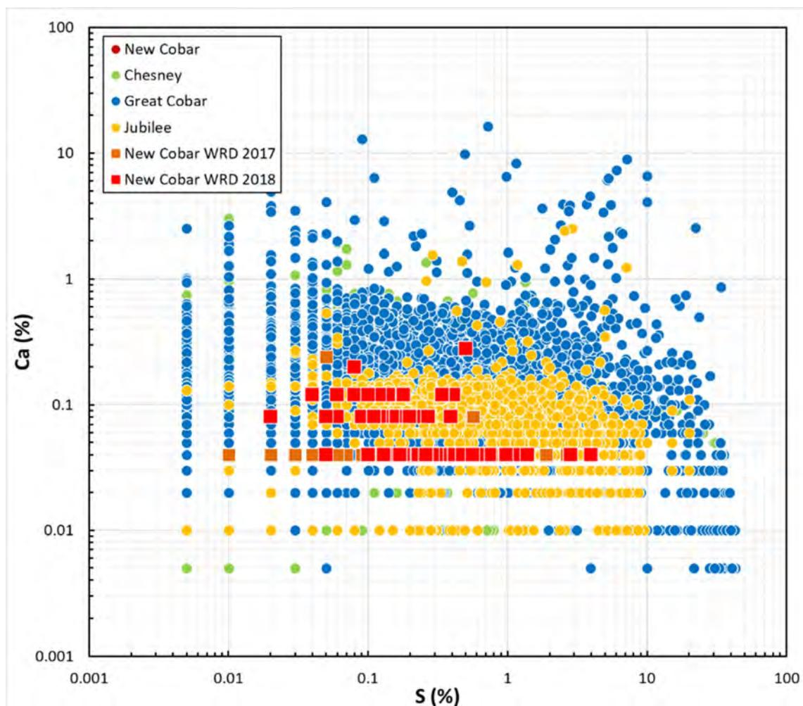
**Figure 3.2** Calcium versus sulfur for New Cobar Complex ore body assays and waste rock
