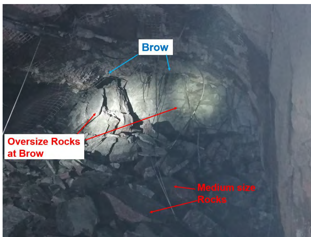
Figure 3.29. Example scenario showing a drawpoint photo of the stope shown in Figure 3.27 and Figure 3.28 in 2020 showing major stope overbreak and dilution due to collapse of the stope hangingwall at another mine with a diminishing central pillar
