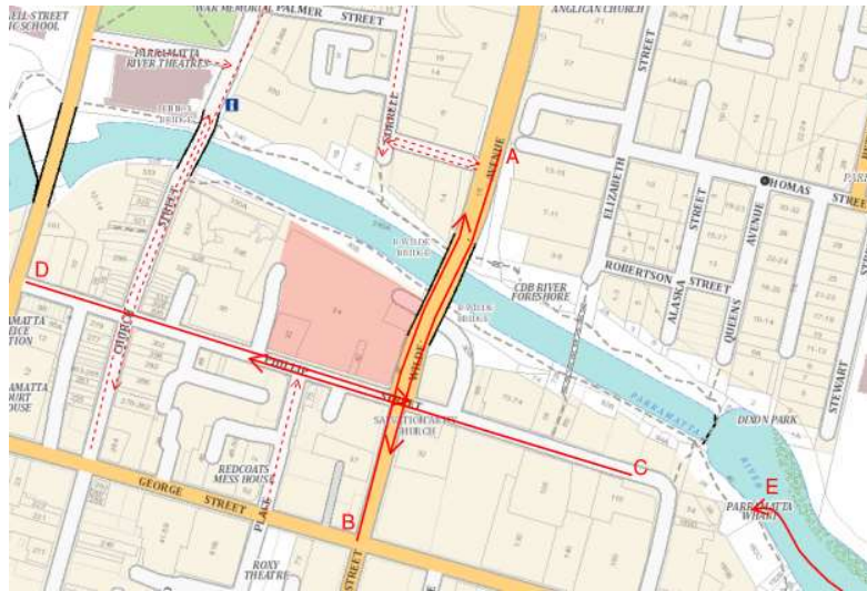
Figure 5: Site map showing observer paths from which glare has been assessed, with the New Powerhouse highlighted in red. Paths dotted in red indicate paths assessed, but not included in report due to negligible glare impact, e.g. New Powerhouse not within field of driver view, or of negligible luminance (less than 500 Cd/m 2 ).
