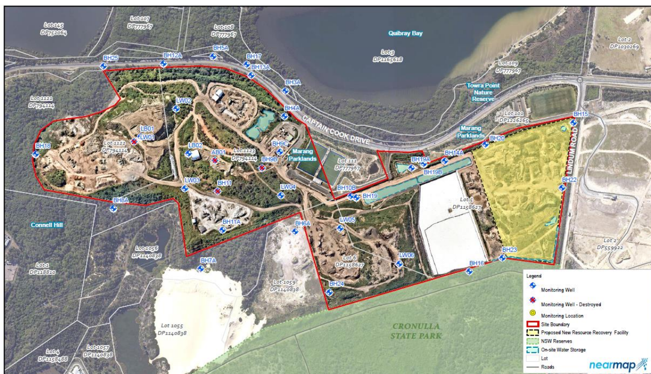
Figure 37 Groundwater and leachate monitoring wells
