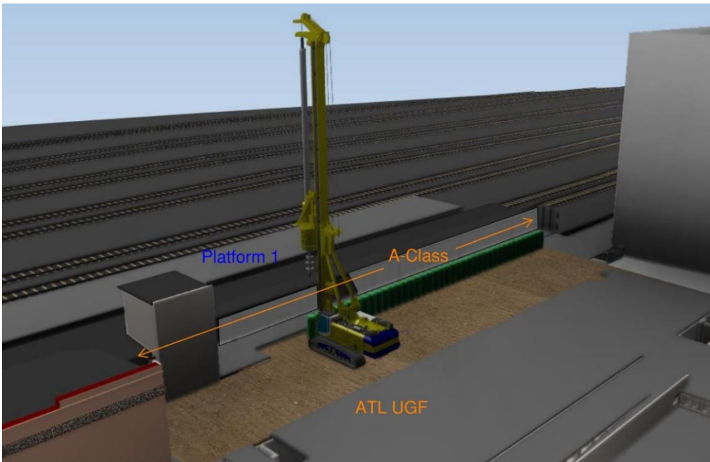
Figure 2-14: Example of piling rig in relation to Platform 1 A-Class Hoarding
