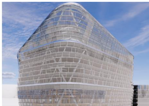
1.5 FIGURE 4 - PROPOSED DESIGN: CROWN EXTERIOR FACADE TO BE FIXED GLAZING - VIEW FROM NORTH WEST
