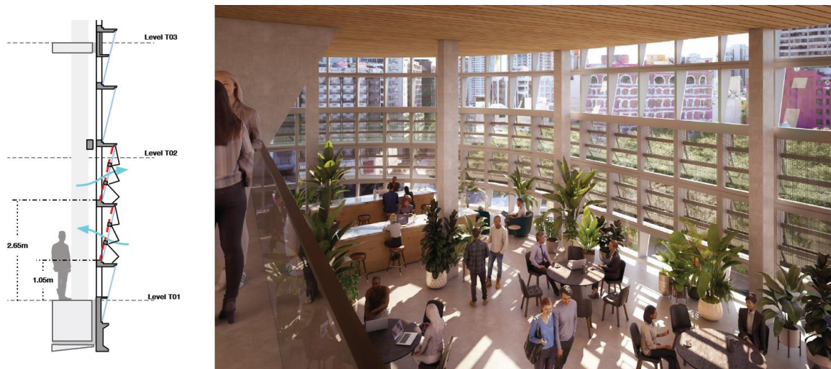
Figure 5 Section and interior view showing proposed awning windows on Level 1
