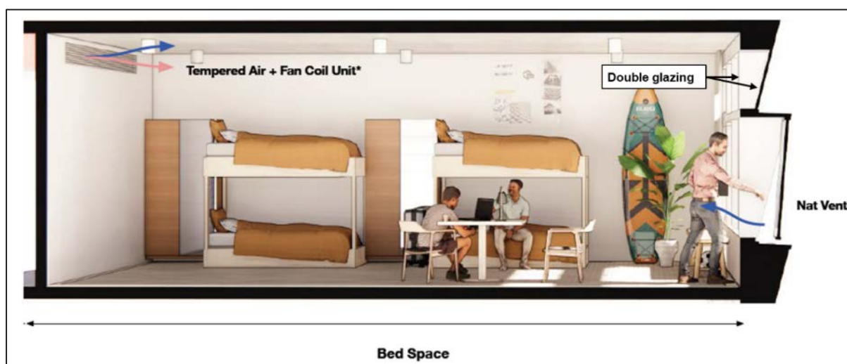
Figure 56 | Mixed natural / mechanical ventilation for YHA rooms (Source: Applicant's RtS)
