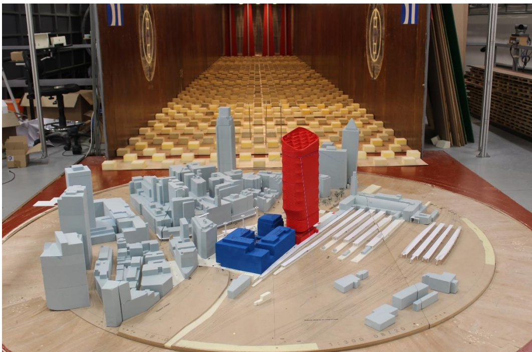
Image 3: View from the south of the Atlassian Central Development with Existing Surrounding Buildings, Local Landscaping and Wind Mitigation Measures in the wind tunnel
