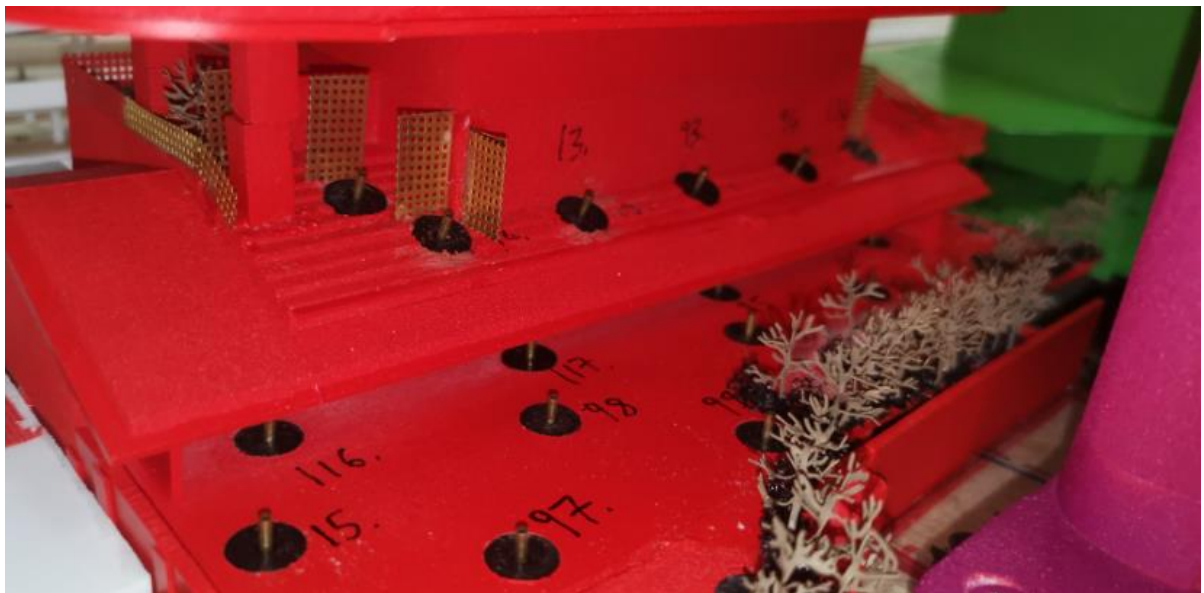
Image 8c: Vertical porous screens (5m in height, 3m wide), placed on the podium around the northern corners
