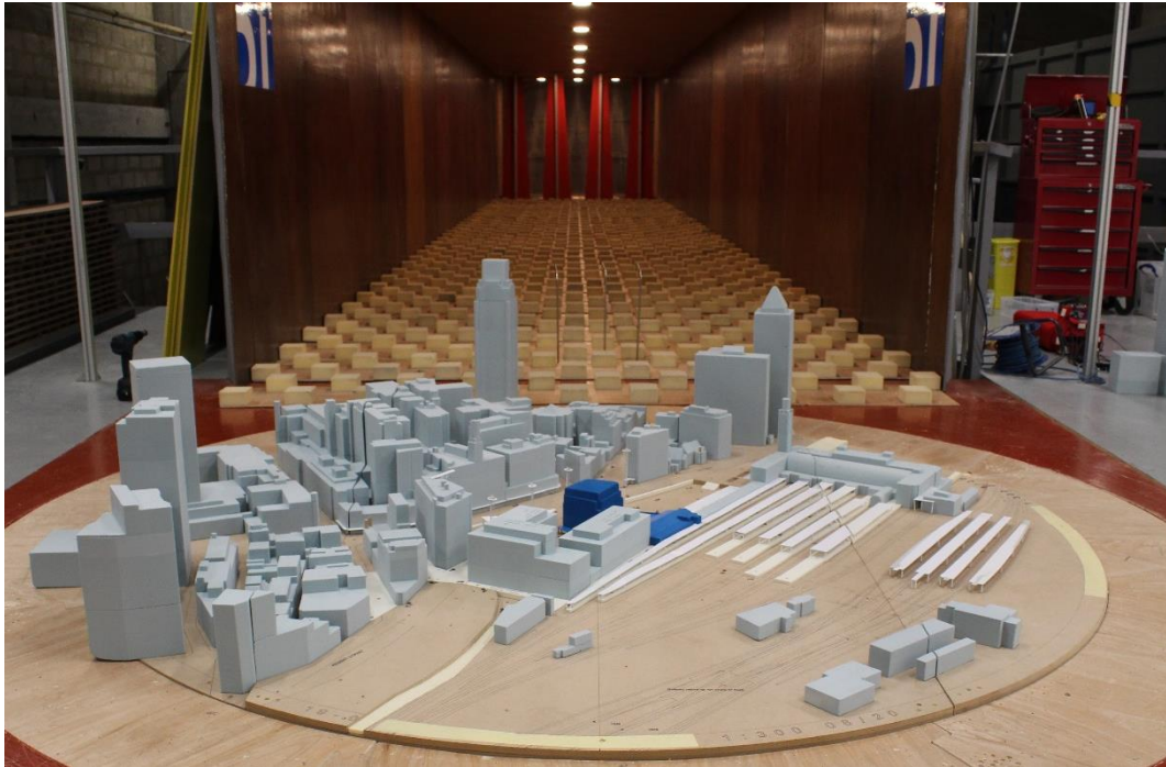
Image 2: View from the south of the Existing Site with Existing Surrounding Buildings in the wind tunnel
