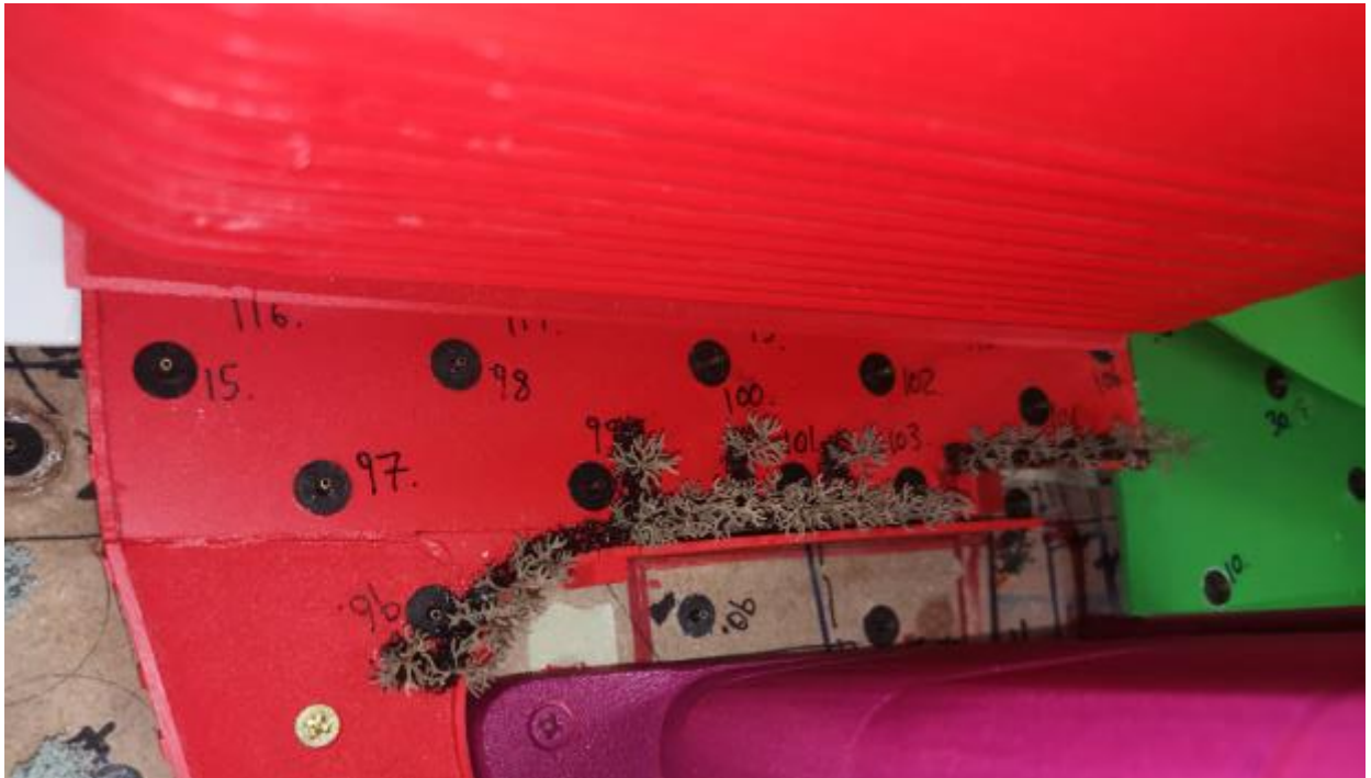
Image 8d: Deciduous trees 6m tall with shrubs 1.5m tall placed underneath along the lower part of the podium
