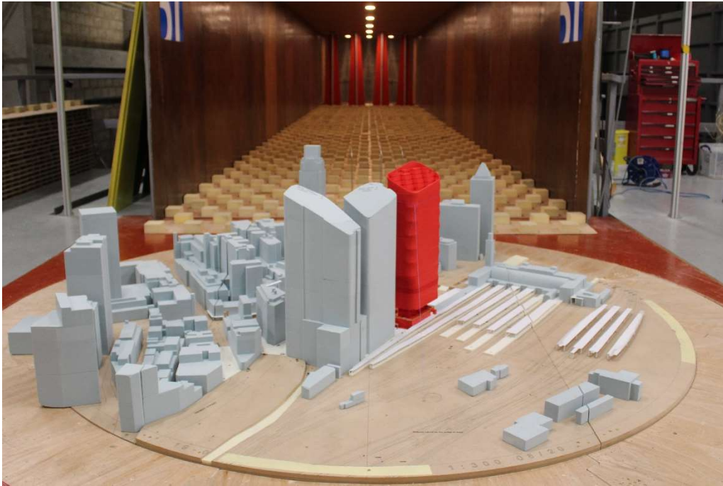
Figure 4: View from the south of the Proposed Development and Dexu/Fraser massing envelope with Existing Surrounding Buildings in the wind tunnel
