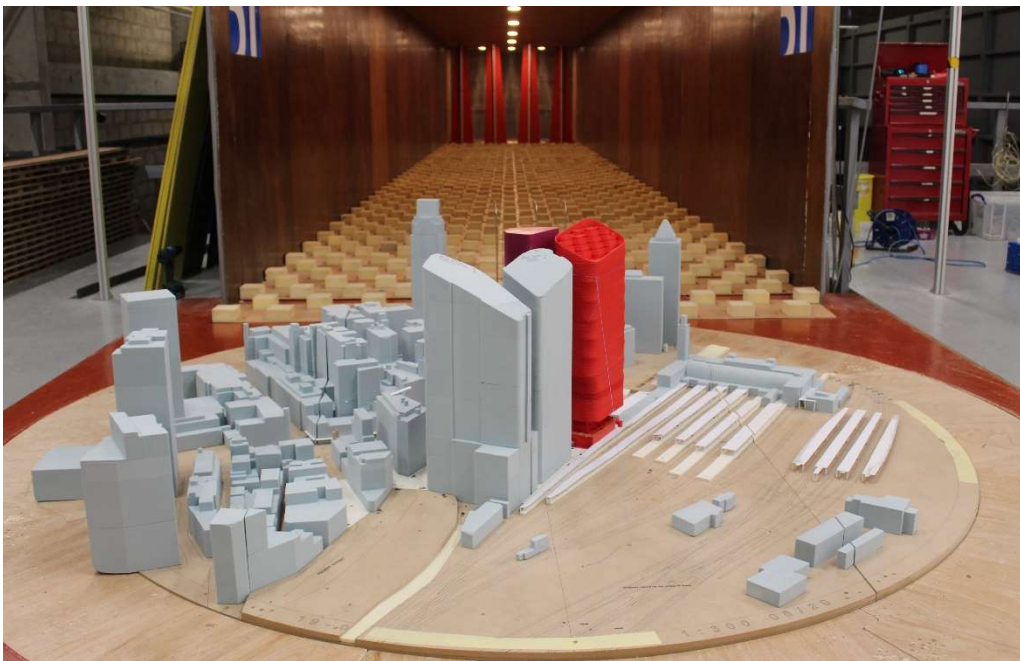
Figure 5: View from the south of the proposed development, Dexu/Fraser and Toga massing envelopes with Existing Surrounding Buildings in the wind tunnel
