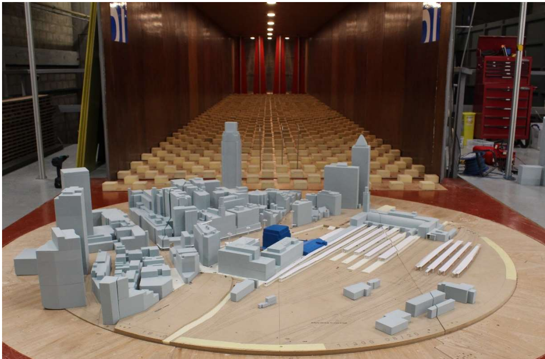
Figure 2: View from the south of the Existing Site with Existing Surrounding Buildings in the wind tunnel
