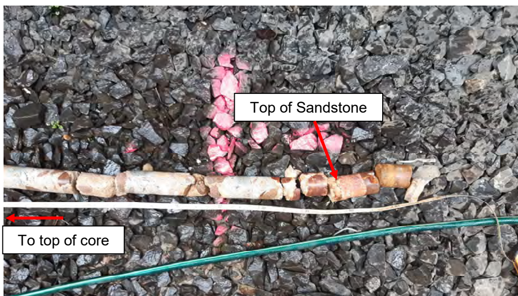
Photo D4 – View of concrete core from Borehole BH105 (below about 5.6 m depth), showing concrete with high strength sandstone inclusions (cyclopean concrete) overlying weathered fine to medium grained sandstone.
