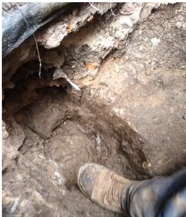
Photo D1 – View within borehole BH101, showing the sand and gravel fill encountered at shallow depth below the rail ballast / ground surface level between the rail carriage dormitories.
