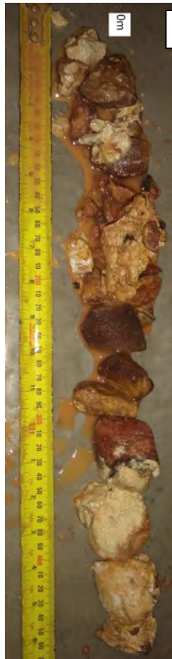
Photo W3 – View of core obtained from Borehole W3. Weathered sandstone was encountered from the start of the borehole.
