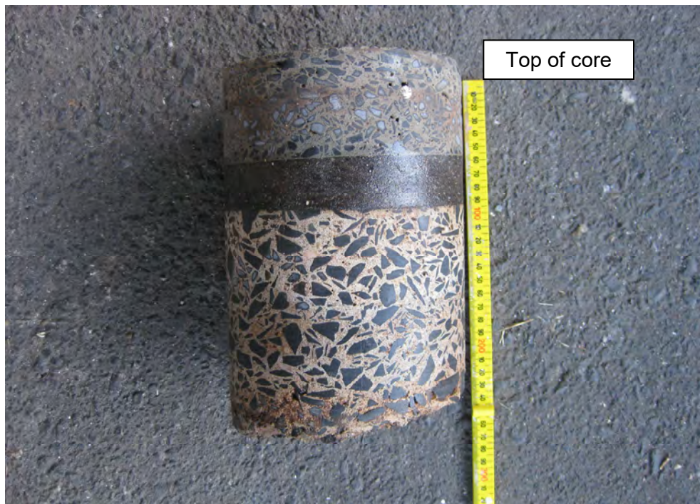
Photo D1 – View of concrete core from Borehole BH6, showing two separate concrete slabs separated by a 30 mm thick asphalt layer. Reinforcement steel (8 mm diameter) was encountered in the lower concrete slab.
