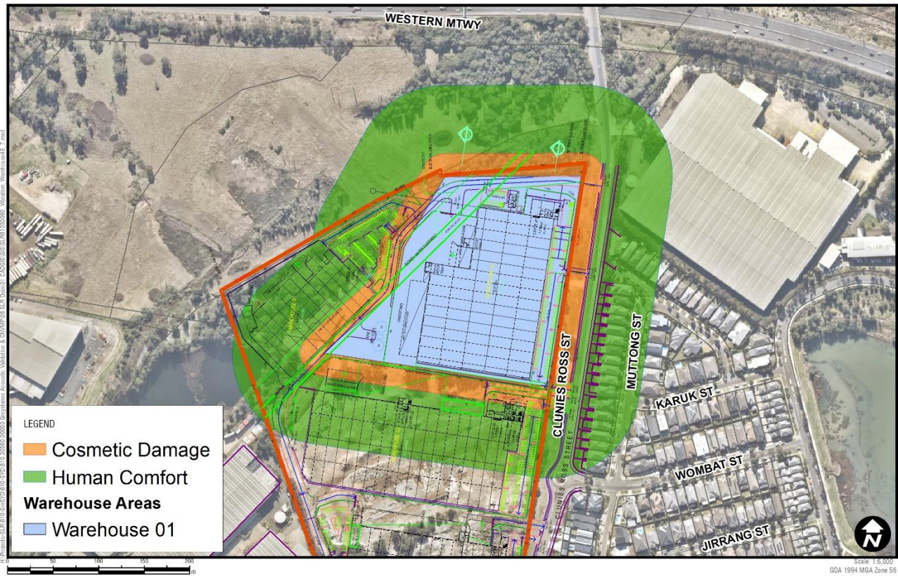
Figure 3 Construction Vibration Assessment – Warehouse 01
