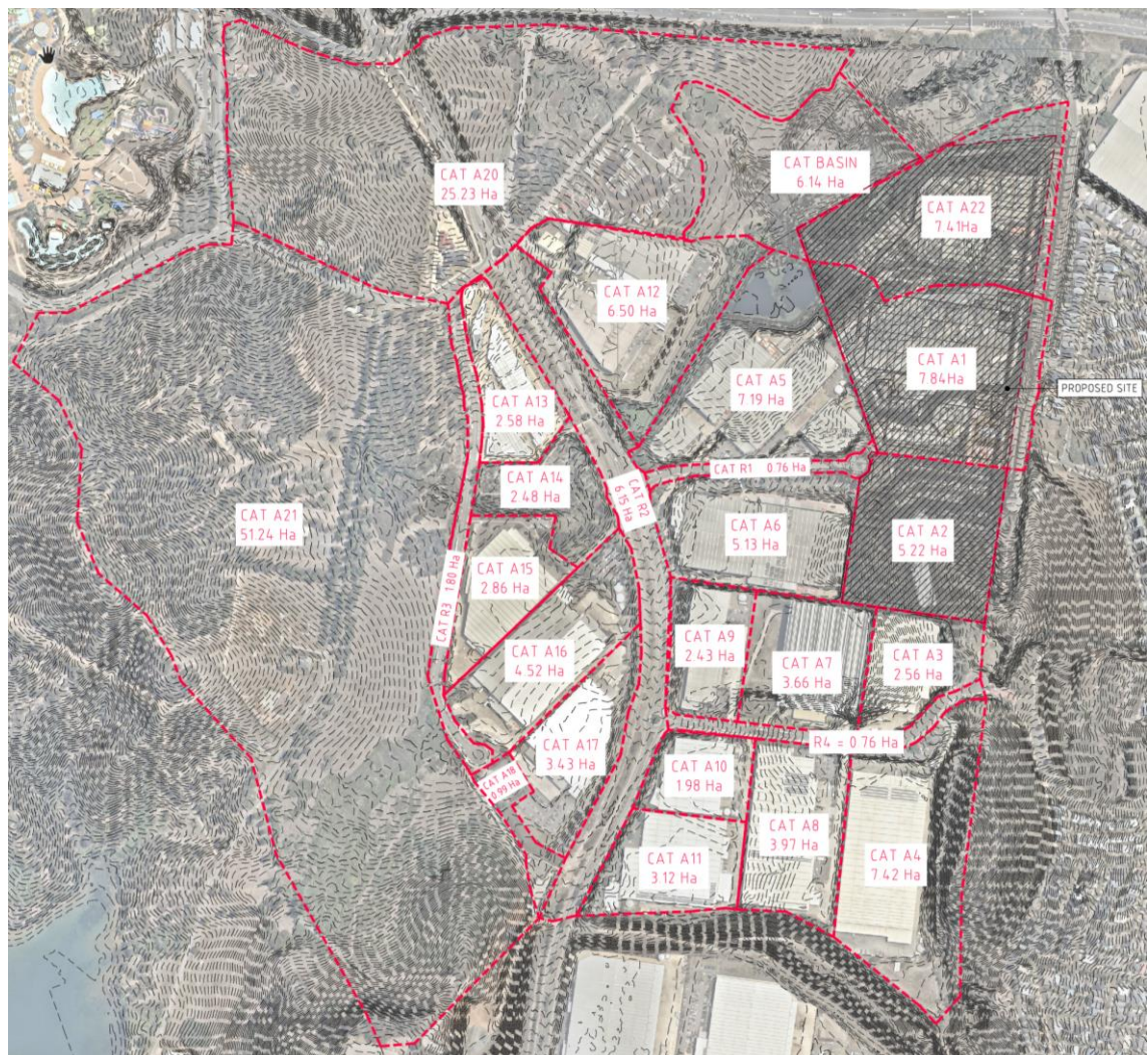
Figure 6.1. Regional Detention System Catchment Layout
