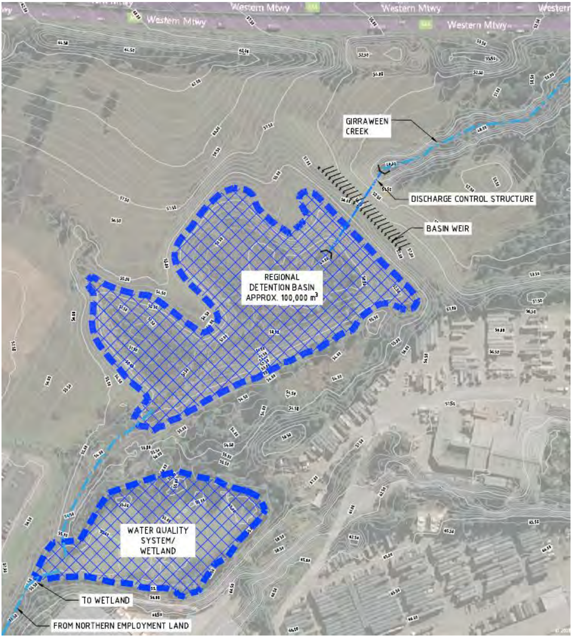
Figure 5.4. As Constructed Stormwater Management Systems
