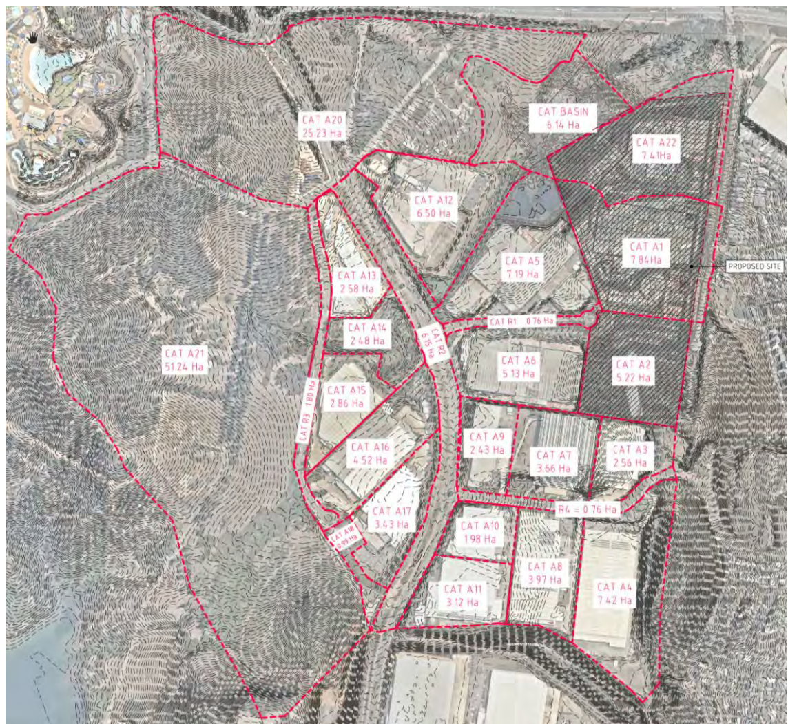
Figure 6.1. Regional Detention System Catchment Layout
