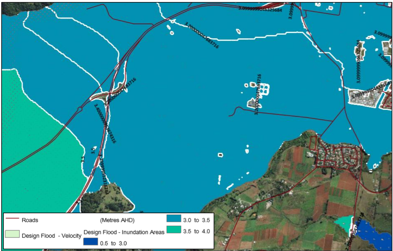
Figure 3.1 Tweed DCP Design Flood Level Maps (Courtesy: TSC)
