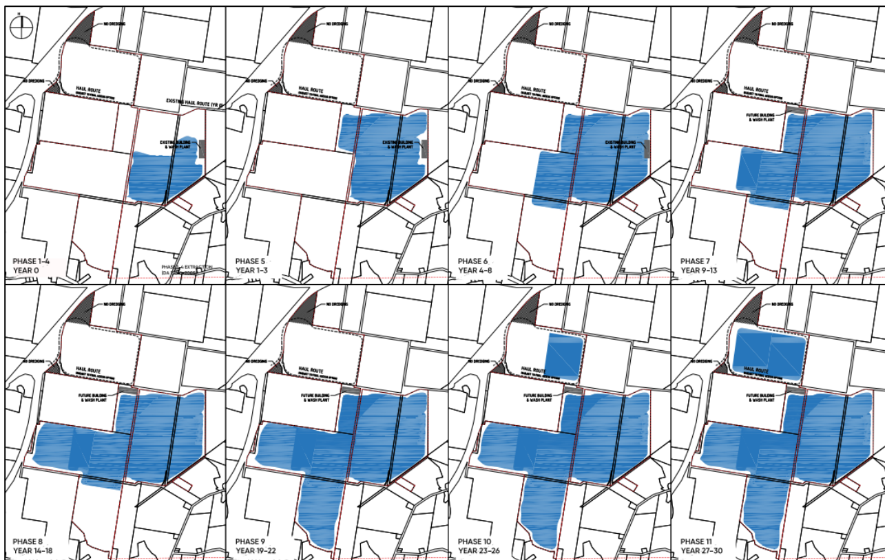
Figure 2.2 Proposed Site Phasing Layout (Zone, 2021)
