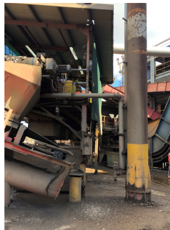
FH27 blocked by debris
