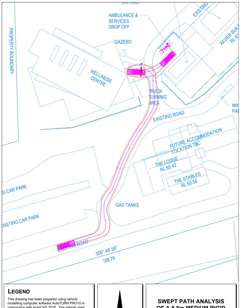
This drawing has been prepared using vehicle modelling computer software AutoTURN PRO10 in conjunction with AutoCAD 2018. The vehicle used is based upon vehicle data provided by Austroads and incorporates a reasonable degree of tolerance. However, it is not possible to account for all vehicle types/characteristics and/or driver ability.
