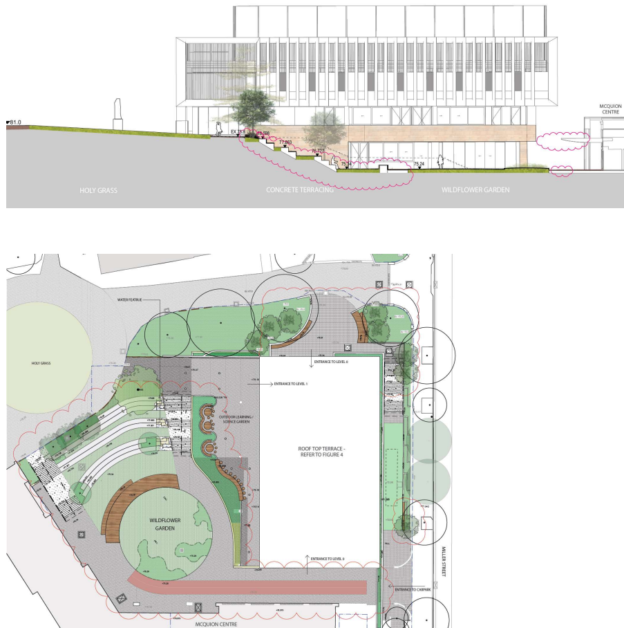
Figure 9 - The section and plan landscape drawings, with the modified areas clouded in red. (Source: Spackman Mossop Michaels)
