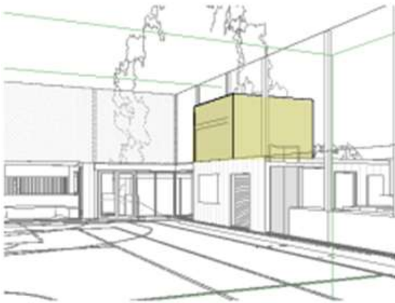
OPTION C: ENCLOSED EXHAUST PIPES (750MM ABOVE THE HEIGHT OF THE LIFT OVERRUN) VIEW FROM THE ROOFTOP
