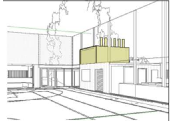
OPTION A: PARTIALLY ENCLOSED EXHAUST PIPES (TO THE HEIGHT OF THE LIFT OVERRUN) VIEW FROM THE ROOFTOP
