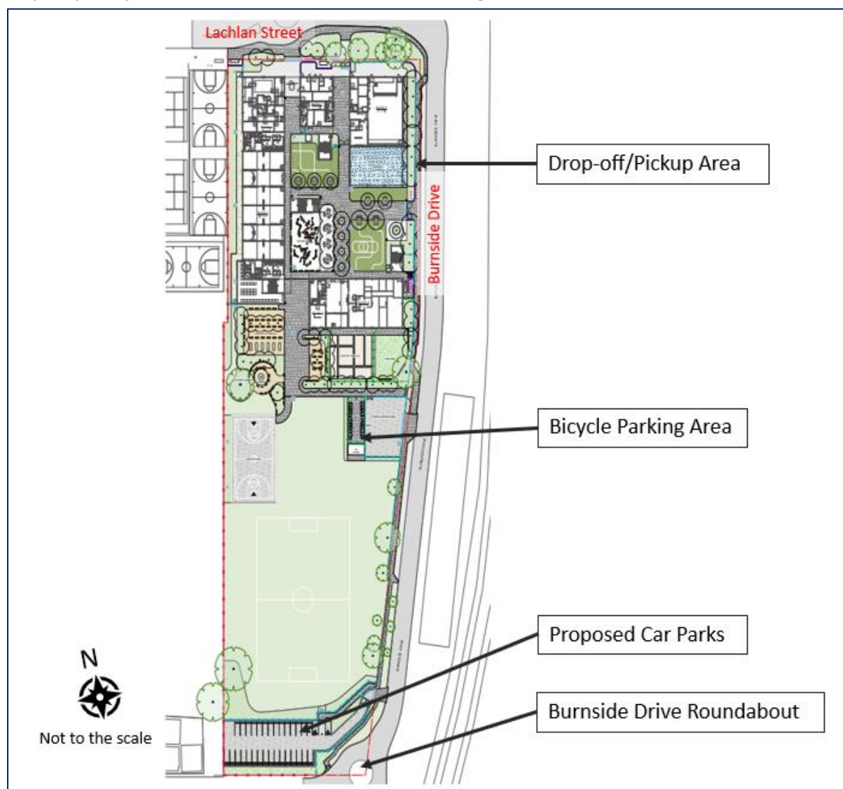
Figure 26 | Proposed traffic infrastructure (Source: Applicant's SRtS 2022)
