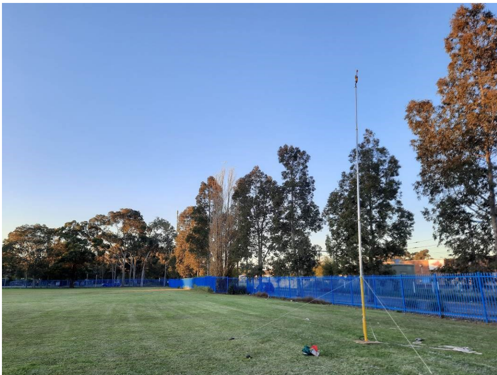
Photo 4. RF Electric Field Measurement Setup at Location 7 of the Proposed New Liverpool Public School
