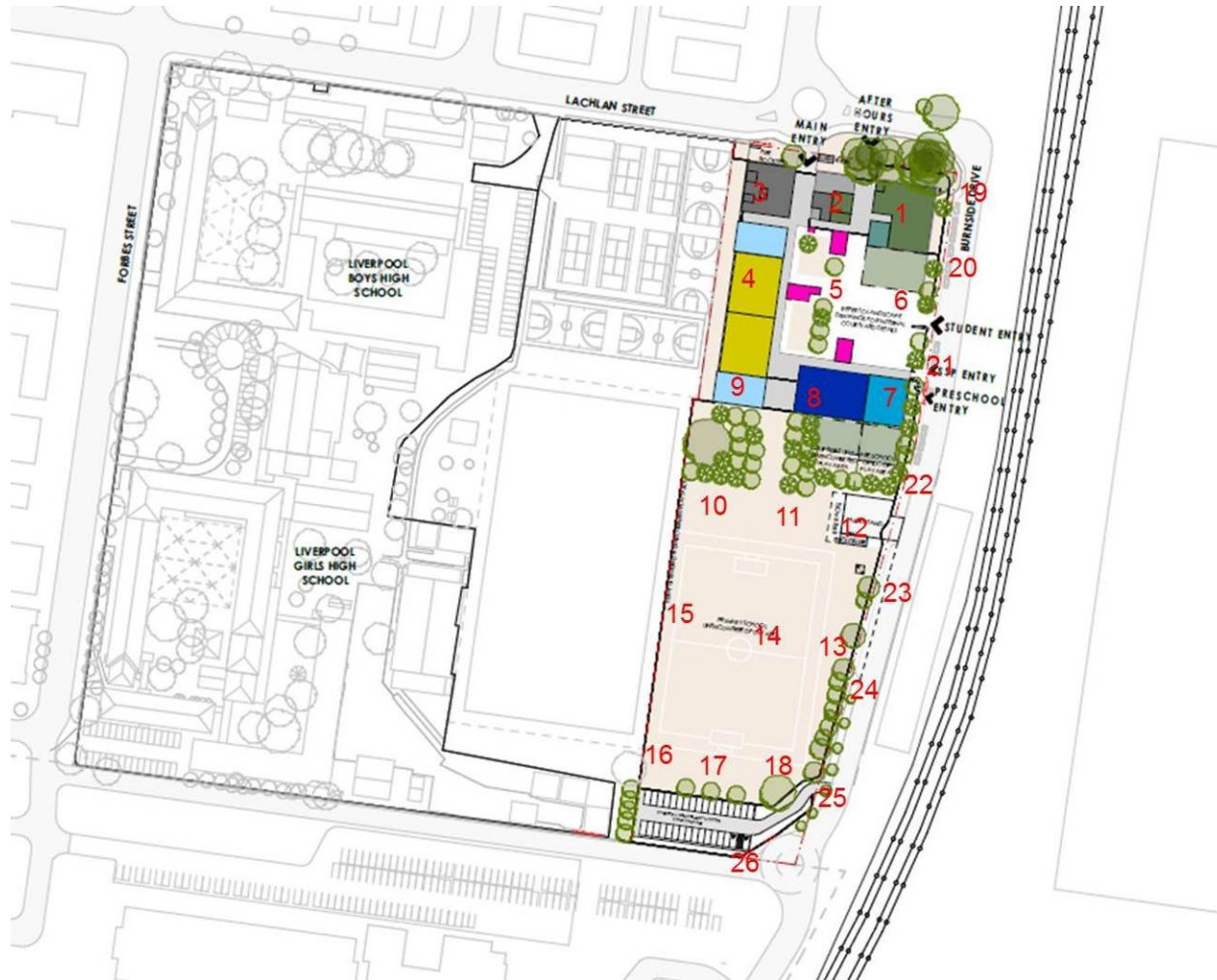
Figure 2. RF Electric Field and Power Frequency Magnetic Field Measurement Locations at the Proposed New Liverpool Public School
