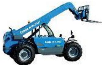
A blue telehandler machine, also known as a telescopic forklift, with a long articulated arm and a bucket-like attachment at the end.                        | All-terrain telescopic forklift style machine which can be used for loading and unloading of materials from trucks, picking and carrying materials to workfronts and lifting materials for installation. |               |
