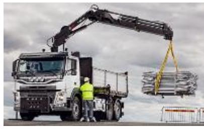
A white delivery truck equipped with a HIAB crane. The crane is extended, lifting a large metal structure, possibly a steel beam or panel, from a truck bed. | Delivery truck with a crane mount with the capability of lifting circa 5 tonne will be used for loading and unloading of materials as well as local delivery to workfronts from the laydown area.        |               |
