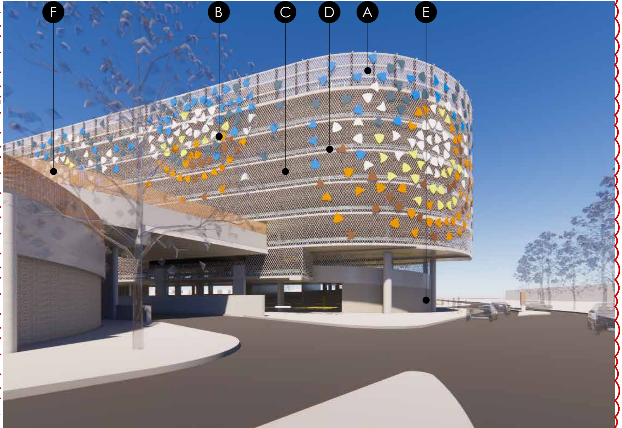
B ALUMINIUM PANELS FIXED TO TENSILE WIRE MESH COLOUR 01 DARK BLUE COLOUR 02 MID BLUE COLOUR 03 LIGHT BLUE COLOUR 04 WHITE COLOUR 05 GREEN COLOUR 06 LIGHT BROWN COLOUR 07 DARK BROWN
