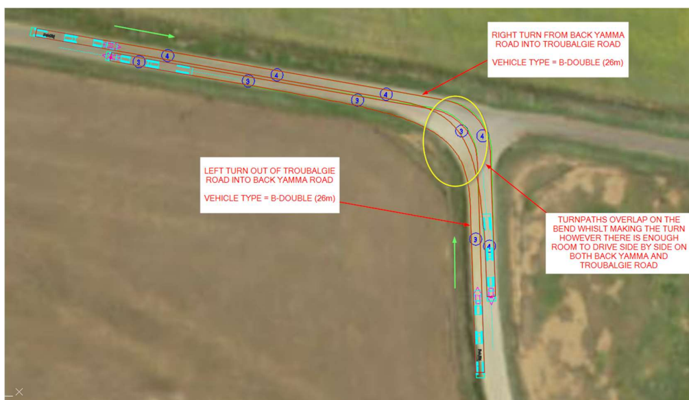
Figure 1-1 Swept path analysis - Back Yamma Road/ Troubalgie Road existing priority intersection
