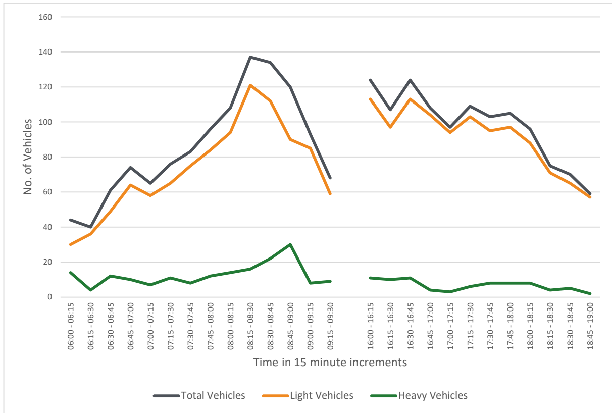
Figure 2-11 Intersection Turning Flows Profile by Vehicle Type at Flint Street/The Escort Way Intersection
