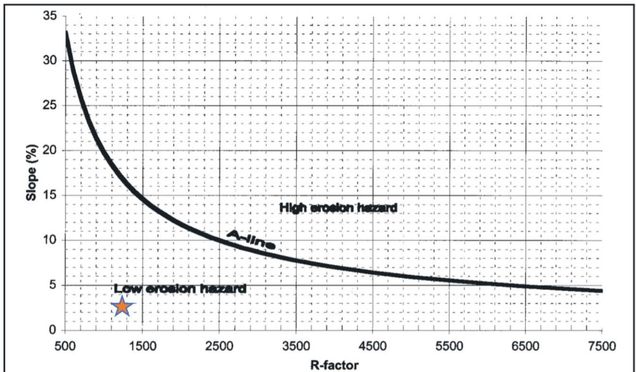
Figure 4-2 Assessment of potential erosion hazard
