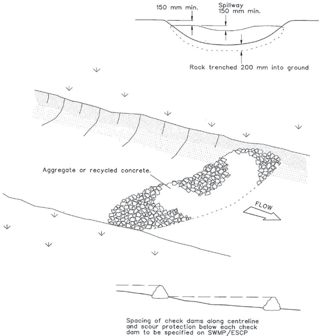
Figure 5-2 A typical rock check dam (Landcom, 2004)
