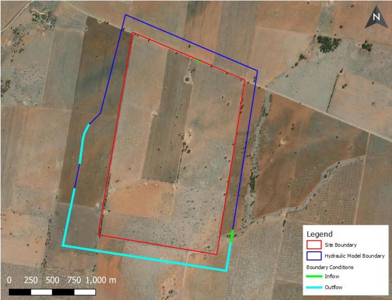
Figure 5-3 Hydraulic modelling of site inflows and out flow (Flooding Risk Impact Assessment Report, SMEC 2020).
