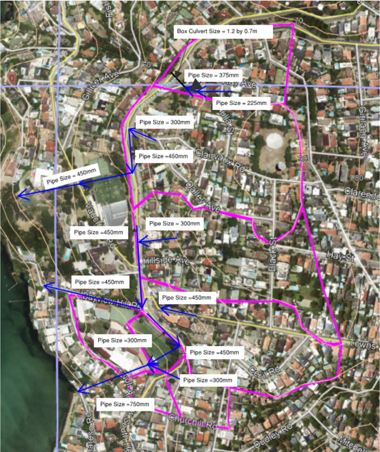
Figure 9 Main Stormwater System included in the DRAINS Model
