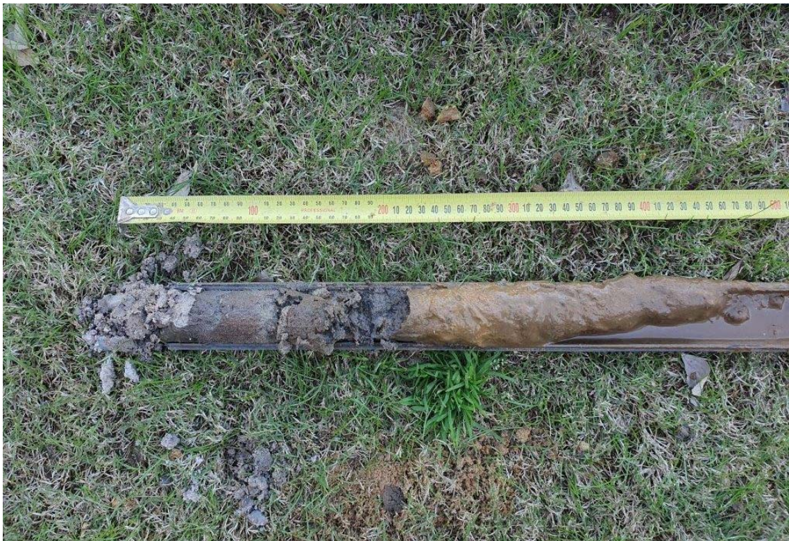
Photo 4 - Standard Penetration Test displaying groundwater in BH103 (12/07/2019)
