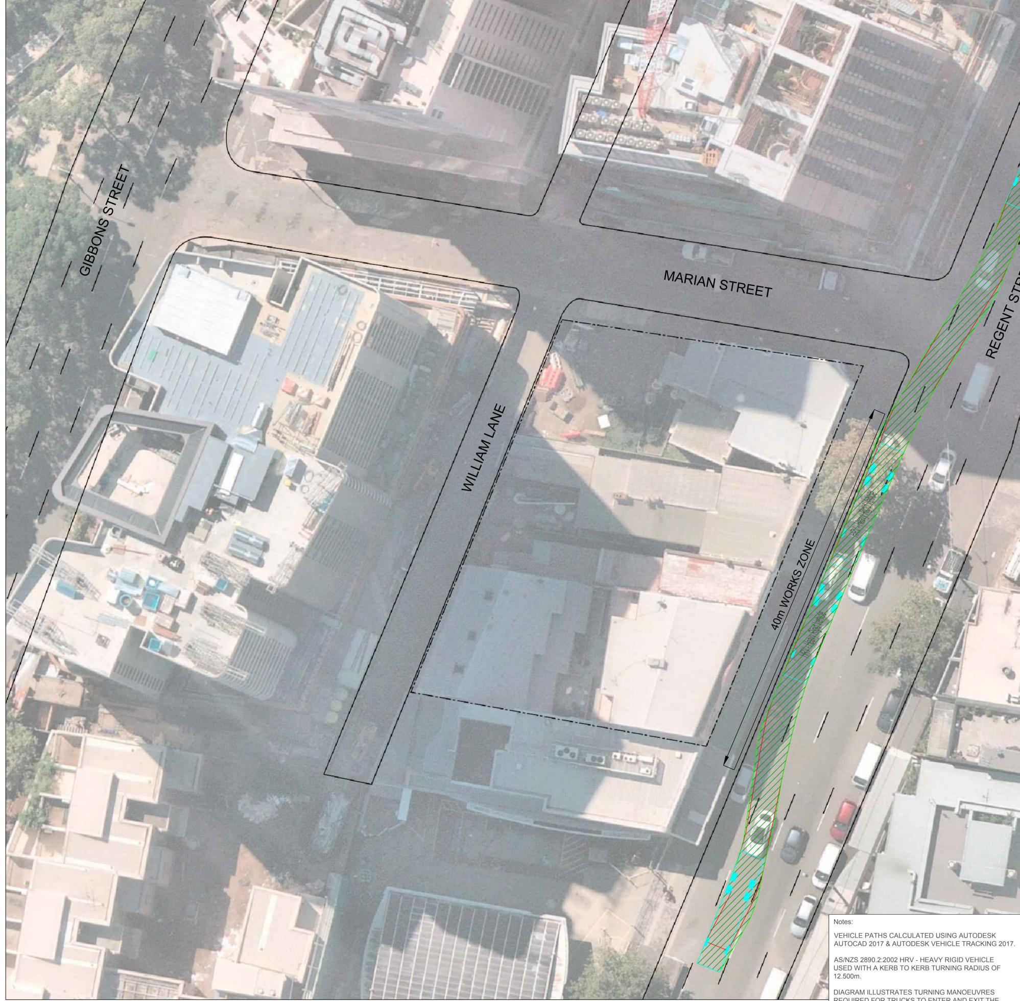
DIAGRAM ILLUSTRATES TURNING MANOEUVRES REQUIRED FOR TRUCKS TO ENTER AND EXIT THE PROPOSED WORKS ZONE ALONG REGENT STREET.
