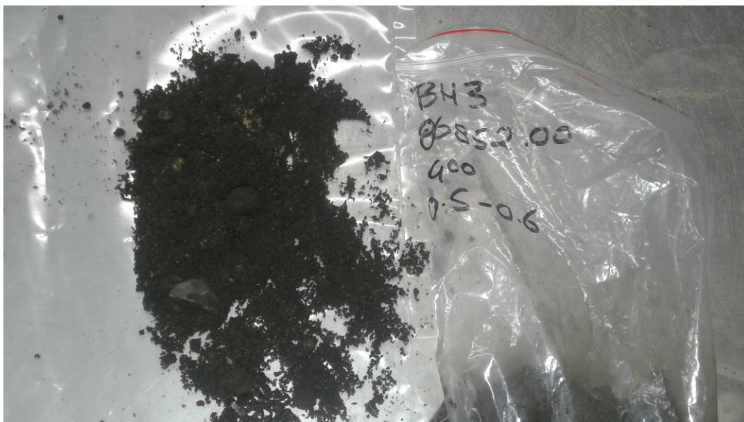
Photograph 9: Ash-containing material in BH3
